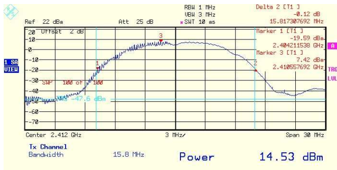
Plot # 55. Output 3 peak power. Lower frequency. 1Mbps rate.
