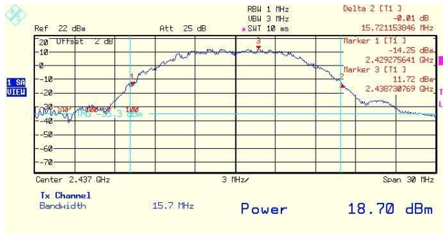
Plot # 71. Output 4 peak power. Middle frequency. 1Mbps rate.
