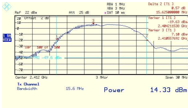
Plot # 31. Output 1 peak power. Lower frequency. 1Mbps rate.
