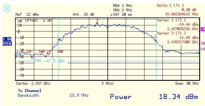
Plot # 35. Output 1 peak power. Middle frequency. 1Mbps rate.
