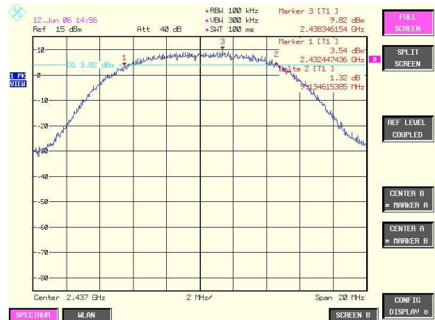
Plot # 24. 6 dB Bandwidth. Middle frequency. 11Mbps rate.
