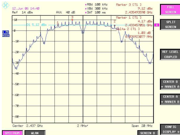
Plot # 23. 6 dB Bandwidth. Middle frequency. 1Mbps rate.
