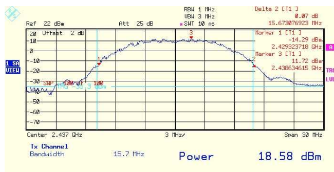
Plot # 47. Output 2 peak power. Middle frequency. 1Mbps rate.
