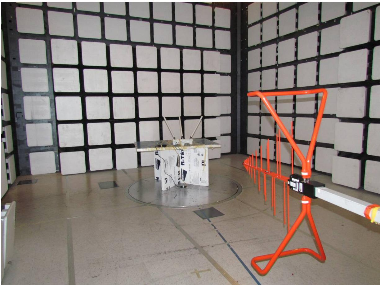
*Radiated Test Setup below 1 GHz SECTOR*
