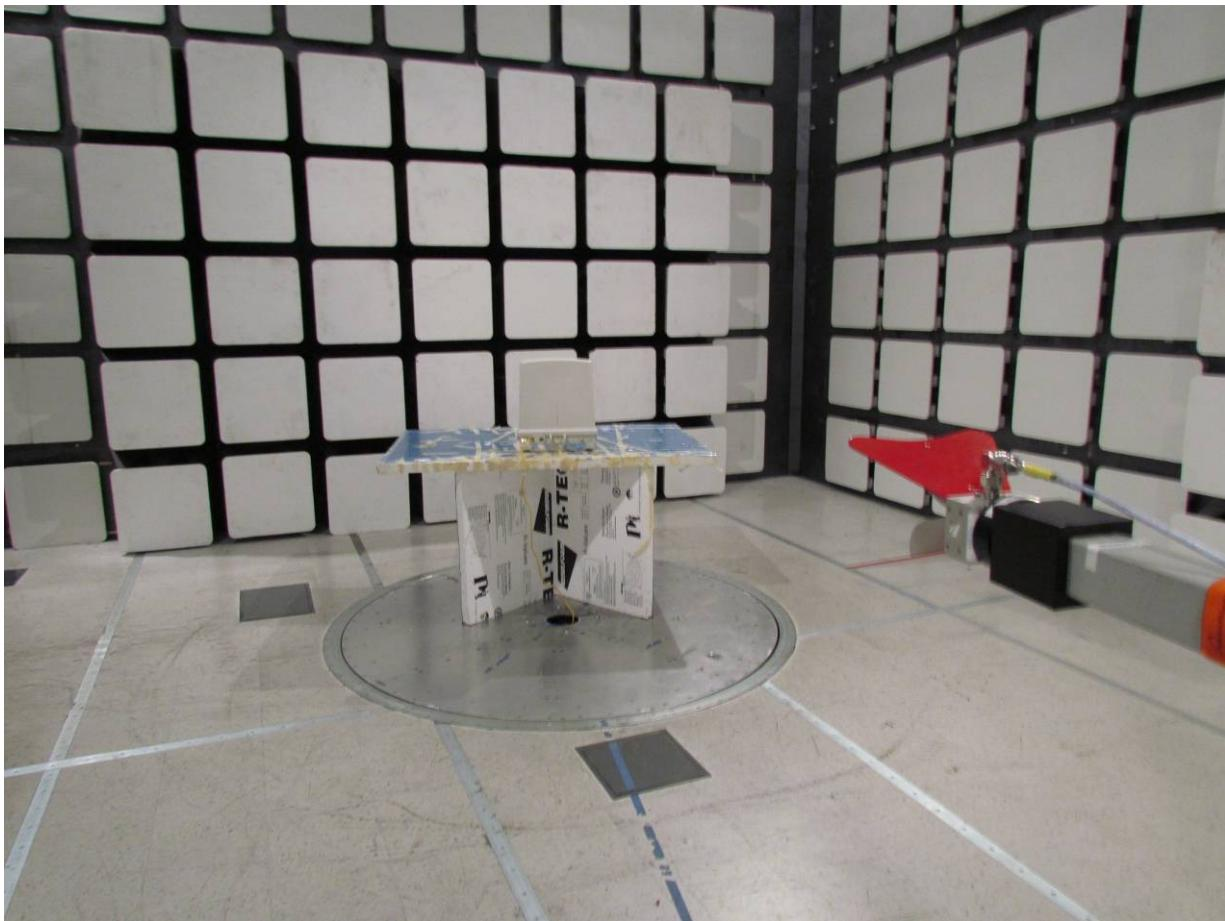
*Radiated Test Setup below 1 GHz OMNI*
