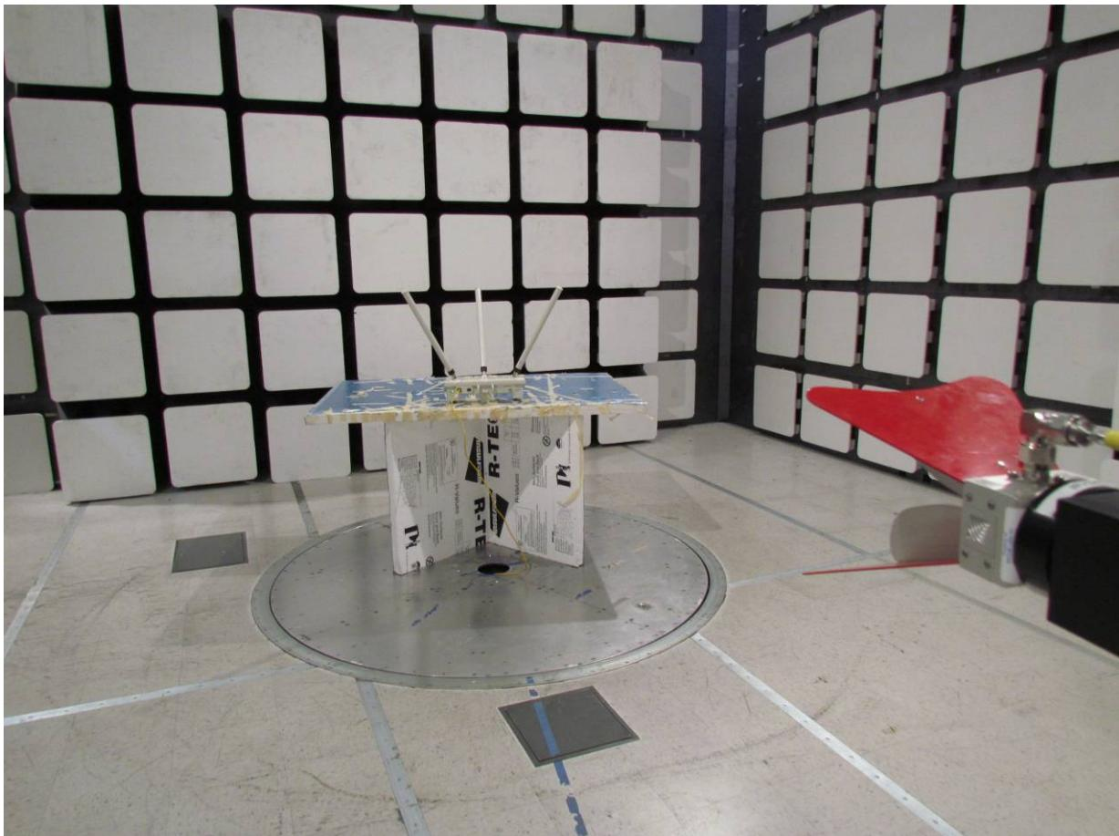
*Radiated Test Setup > 1 GHz SECTOR*
