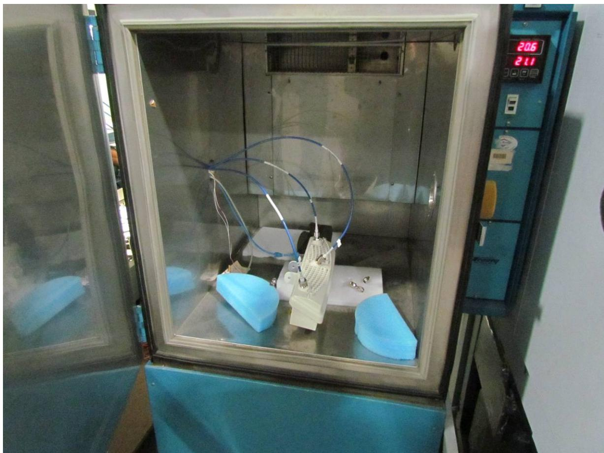
*Radiated Test Setup > 1 GHz OMNI*
