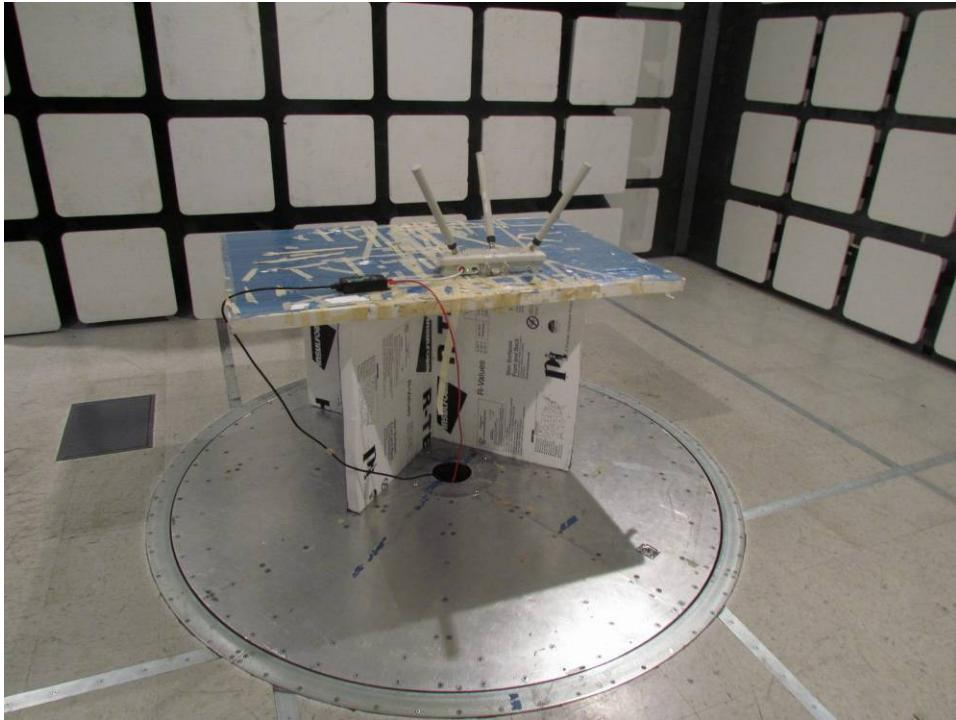
Radiated Test Setup > 1 GHz SECTOR
