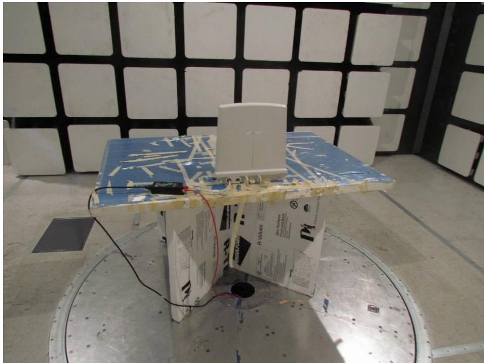
Radiated Test Setup below 1 GHz OMNI
