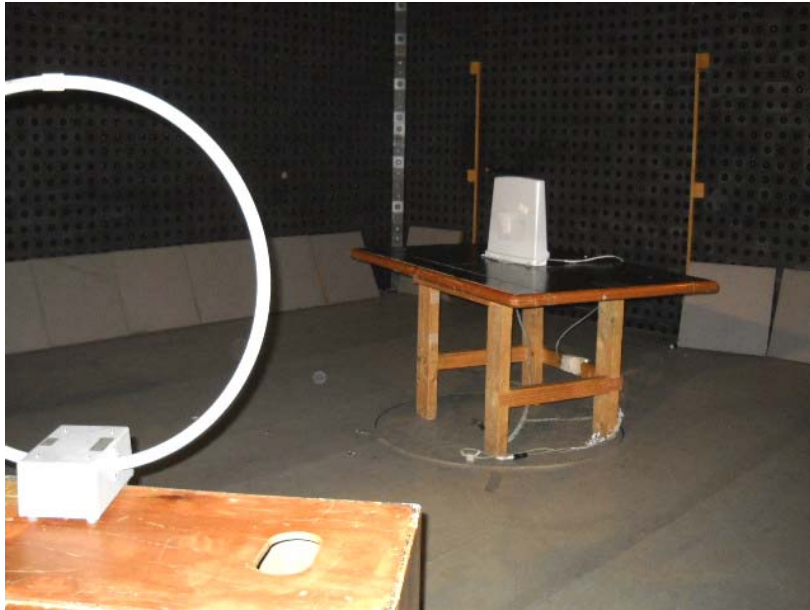
Photograph No.3 Spurious emissions measurement setup in the anechoic chamber below 30 MHz, EUT with sector antenna
