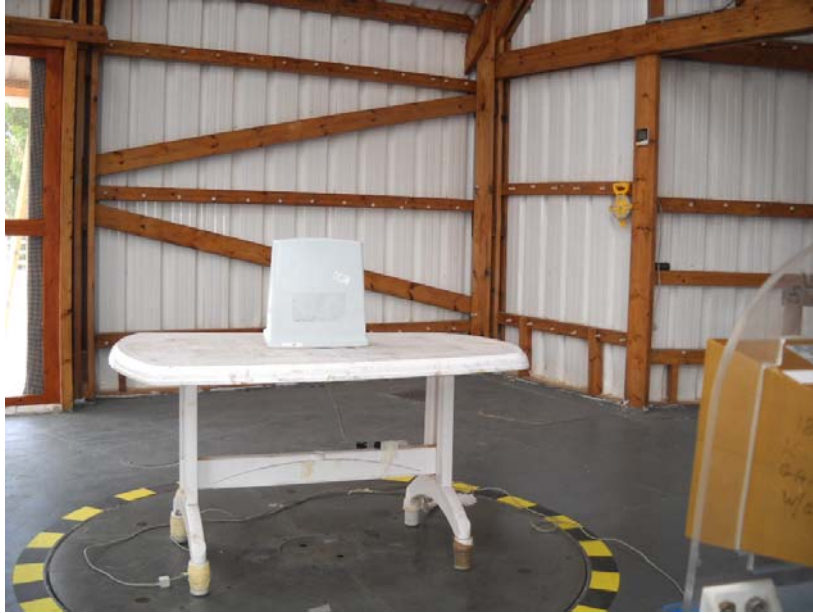
Photograph No.10 Radiated emissions measurement setup at the OATS, EUT with sector antenna
