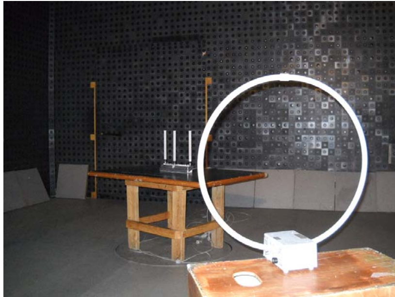
Photograph No.4 Spurious emissions measurement setup in the anechoic chamber below 30 MHz, EUT with OMNI antenna
