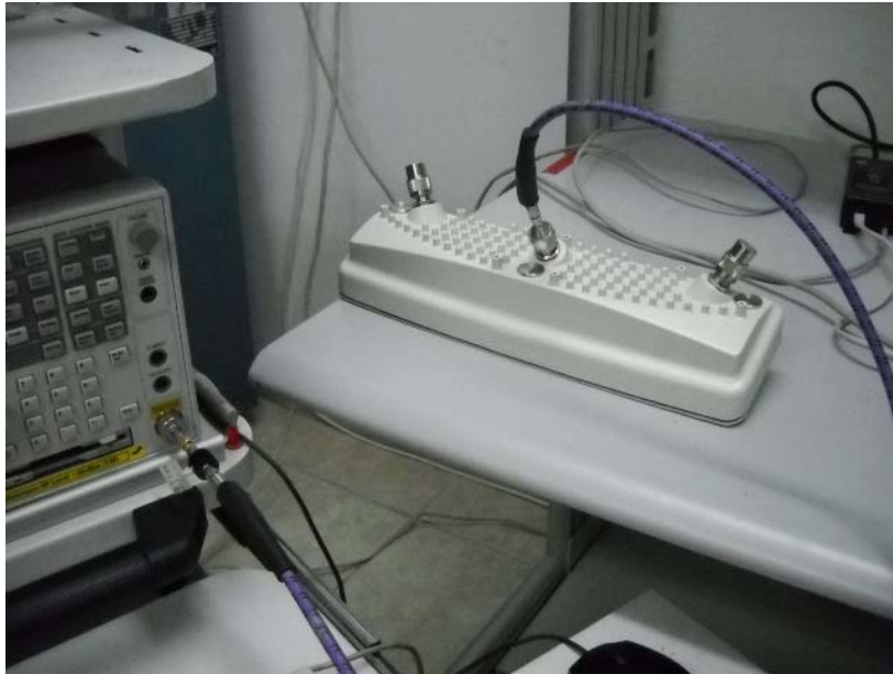
Photograph No.2 Peak power density, occupied bandwidth and conducted spurious emissions measurement setup
