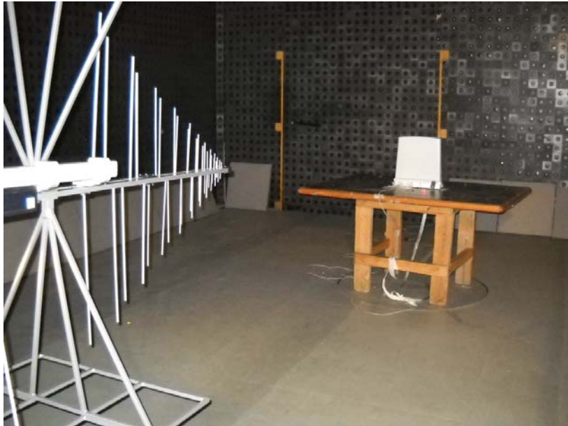
Photograph No.5 Spurious emissions measurement setup in the anechooic chamber in 30 -1000 MHz, EUT with sector antenna
