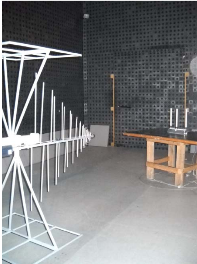
Photograph No.6 Spurious emissions measurement setup in the anechoic chamber in 30 -1000 MHz, EUT with OMNI antenna
