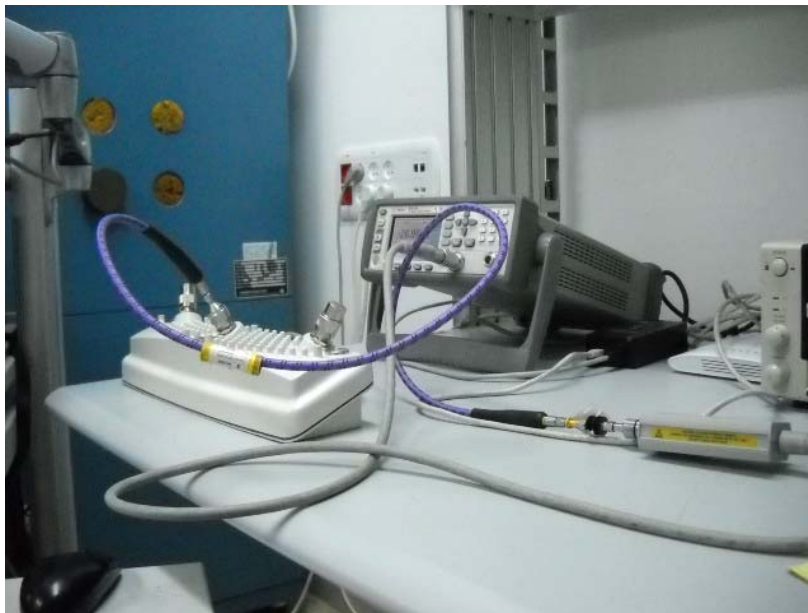
Photograph No.1 Peak output power measurement setup
