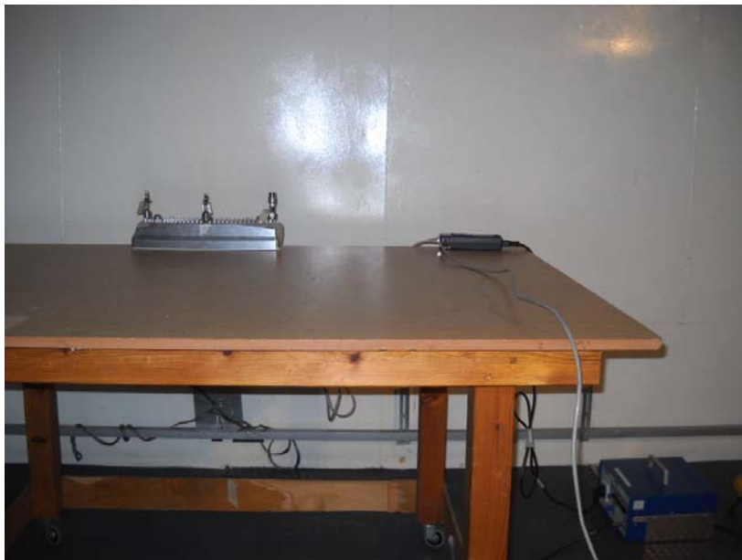
Photograph No.11 Conducted emissions on AC power lines measurement setup
