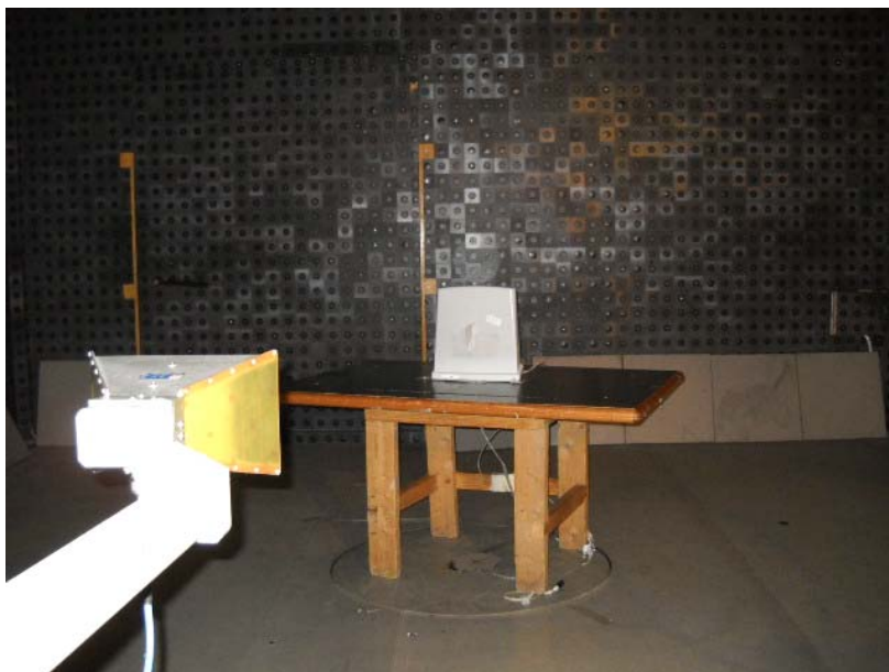
Photograph No.7 Radiated emissions measurement setup in the anechoic chamber above 1000 MHz, EUT with sector antenna
