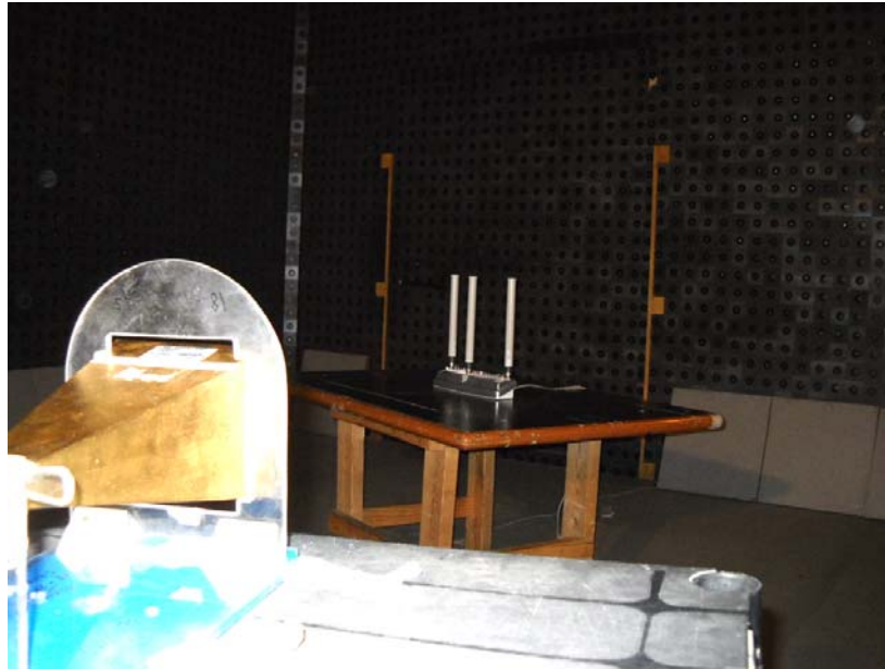
Photograph No.9 Radiated emissions measurement setup in the anechoic chamber above 1000 MHz, EUT with OMNI antenna
