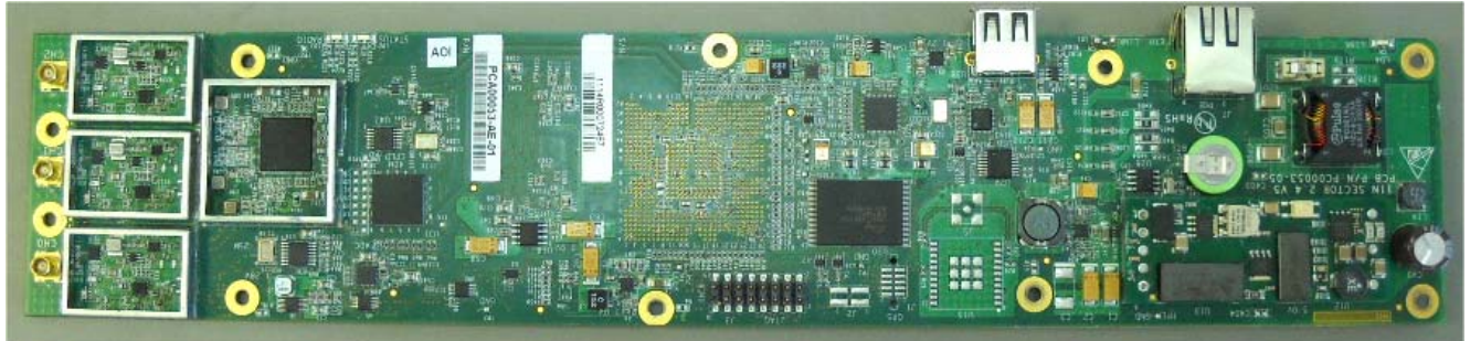
Photograph No.6 WBSn-2400 PCB front view without shields
