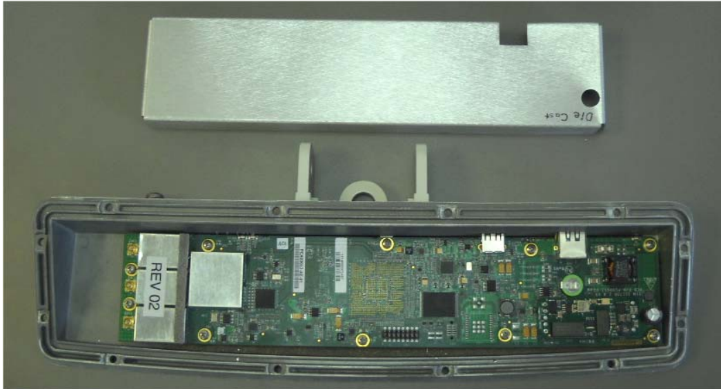
Photograph No.3 WBSn-2400 base station internal view with shield removed
