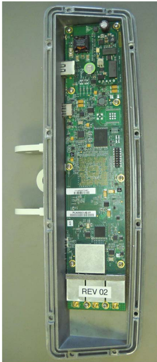
Photograph No.4 WBSn-2400 base station internal view
