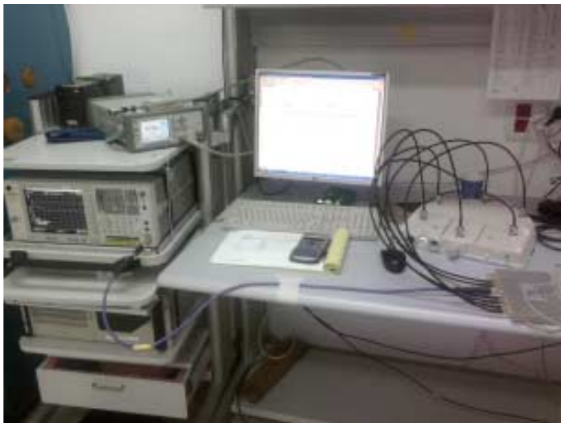
Photograph No.2 Conducted spurious emissions (combined) measurement setup
