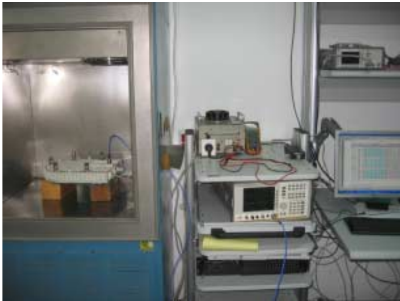
Photograph No.7 Frequency stability measurement setup
