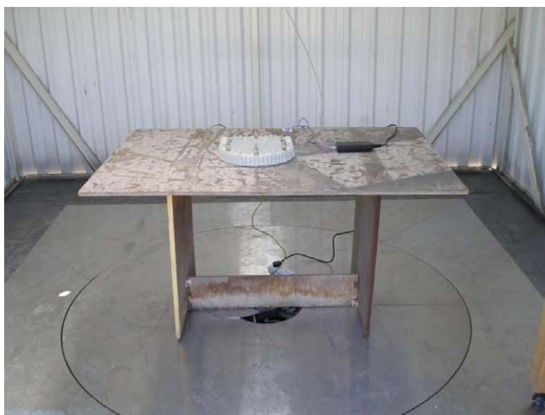
Photo # 1. Radiated emission test set up.
