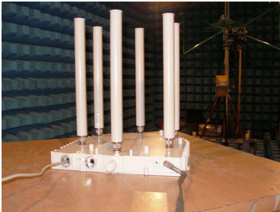
Photo # 3. Radiated emission test on Outdoor Radio Unit: spurious & restricted bands.
