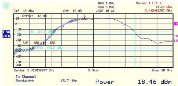
Plot # 168. Output 6 peak power. Lower frequency. 1Mbps rate.
