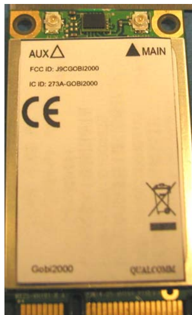
Figure 2 Gobi™2000 Module Label Location
