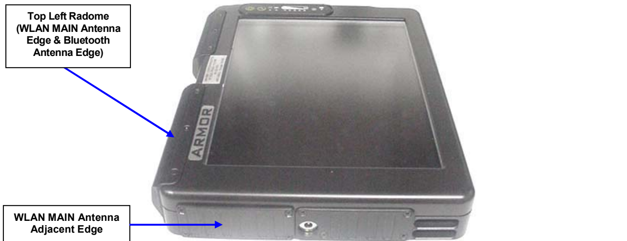
DRS Armor X10 Tablet PC - WLAN MAIN Diversity Antenna Adjacent Edge - "90 Degrees Portrait" (Nylon Case Removed)
