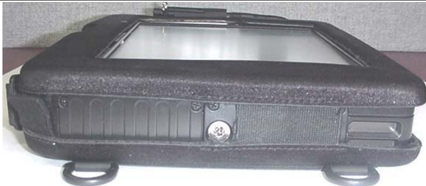
DRS Armor X10 Tablet PC - WLAN MAIN Diversity Antenna Adjacent Edge ("90 Degrees Portrait")
