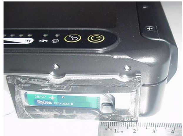
WLAN AUX Diversity Antenna Distance to Adjacent Edge
