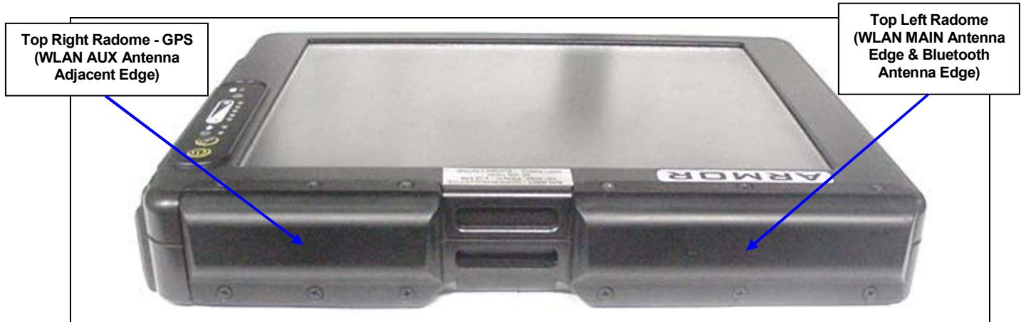
DRS Armor X10 Tablet PC - MAIN Antenna & Bluetooth Antenna Edge - "180 Degrees Landscape" (Nylon Case Removed)
