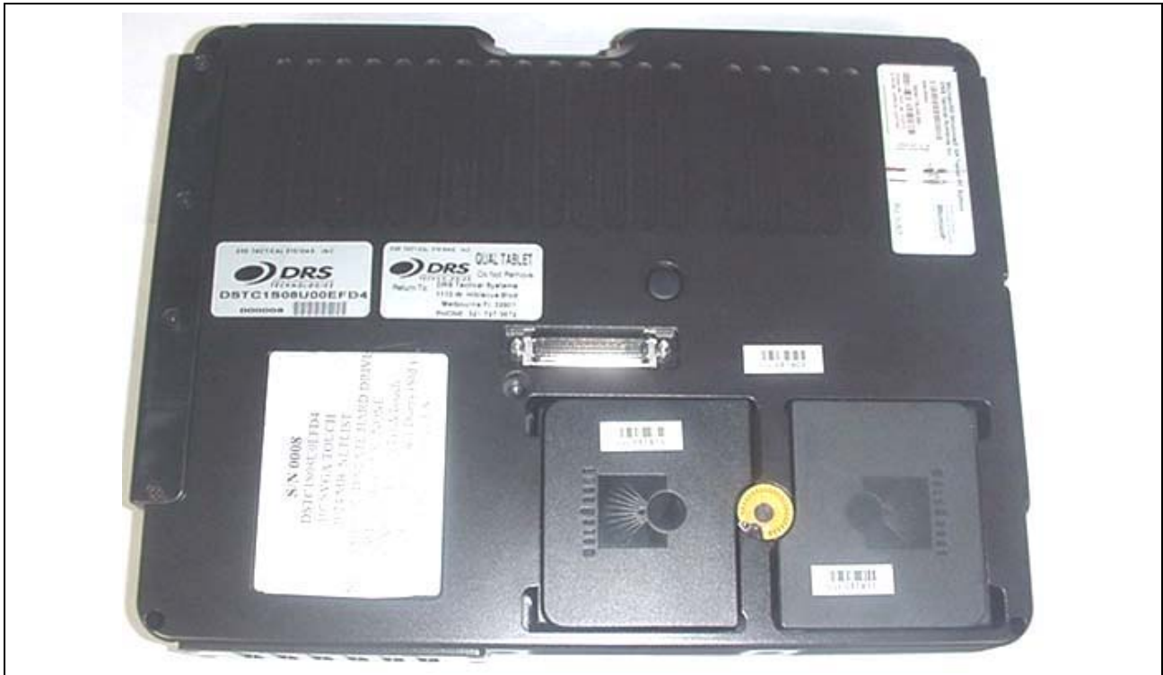
DRS Armor X10 Tablet PC - Bottom Side with Lithium-ion Battery installed (Nylon Case Removed)
