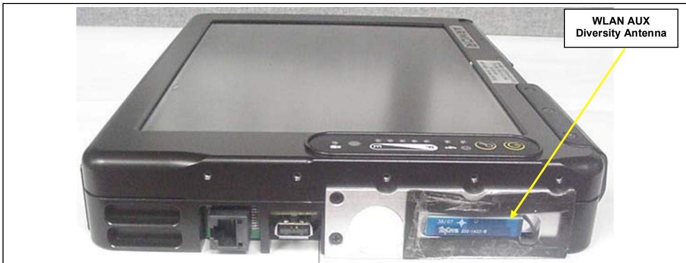
DRS Armor X10 Tablet PC - WLAN AUX Diversity Antenna - "90 Degrees Portrait"
