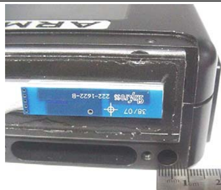
WLAN MAIN Diversity Antenna Distance to Adjacent Edge
