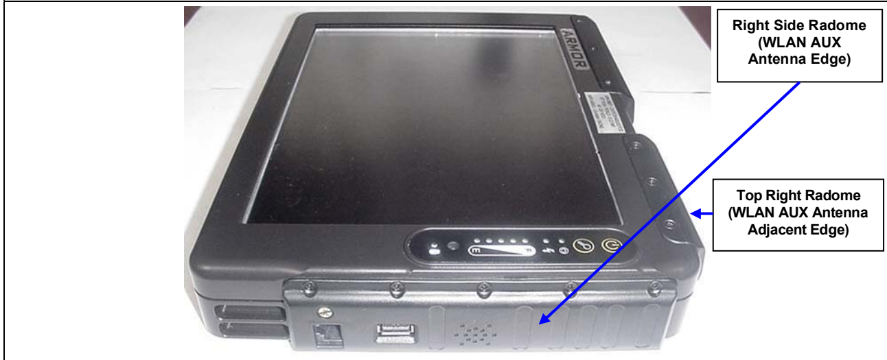
DRS Armor X10 Tablet PC - WLAN AUX Diversity Antenna Edge - "90 Degrees Portrait" (Nylon Case Removed)
