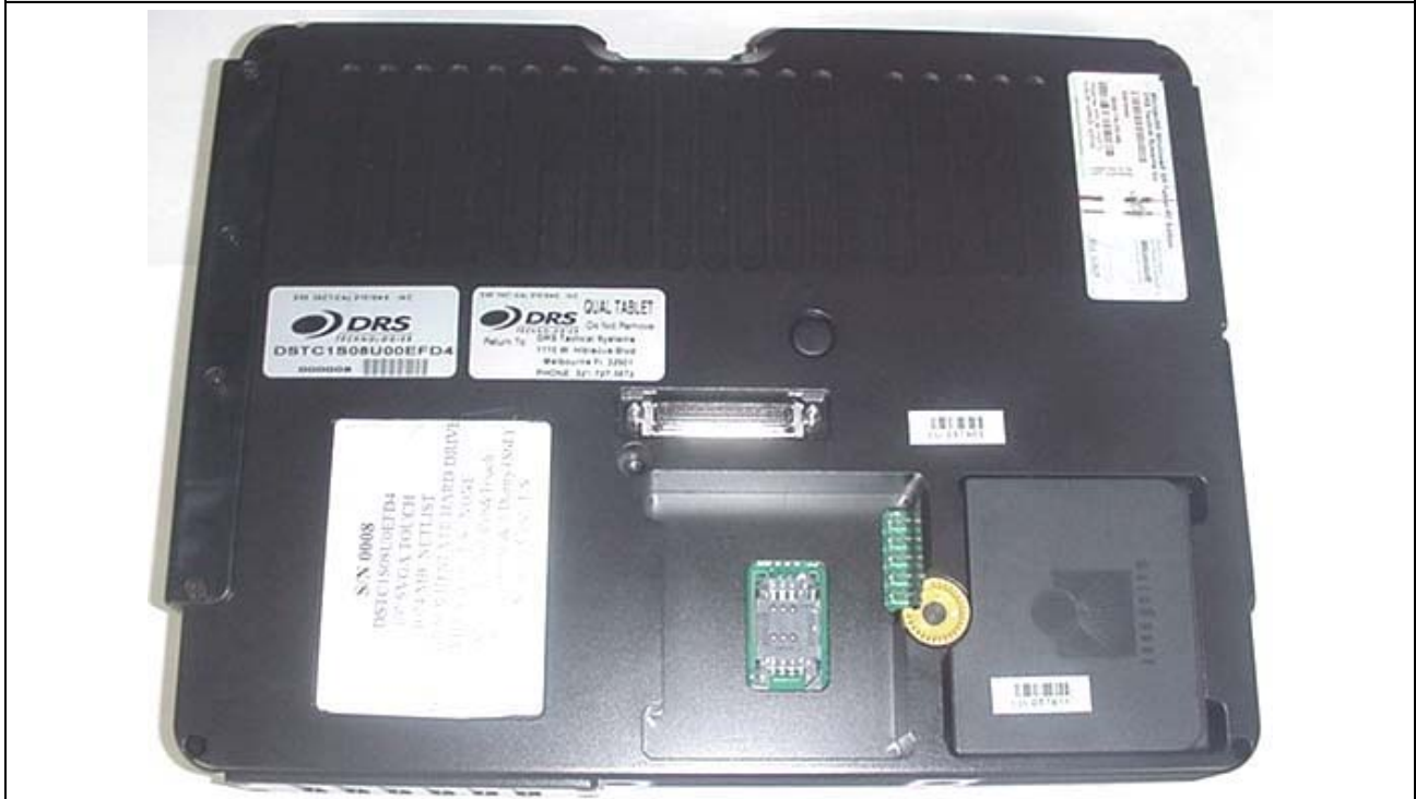
DRS Armor X10 Tablet PC - Bottom Side with Lithium-ion Battery removed (Nylon Case Removed)
