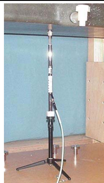
5 GHz Validation Dipole Setup
