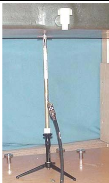
2 GHz Validation Dipole Setup
