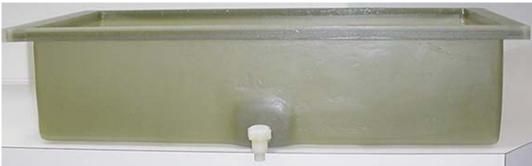
Fiberglass Planar Phantom - Front View
