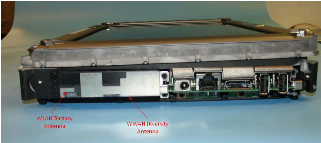
Figure 4 Left View – WWAN Diversity/WLAN Tertiary Antennas
