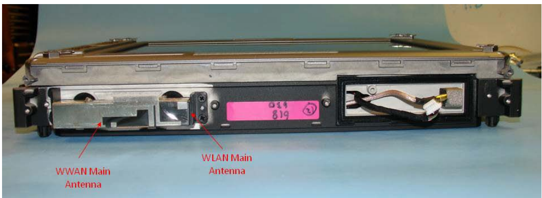
Figure 5 Top View – WWAN Main/ WLAN Main
