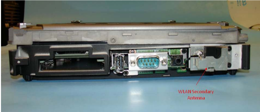
Figure 6 Right View – WLAN Secondary
