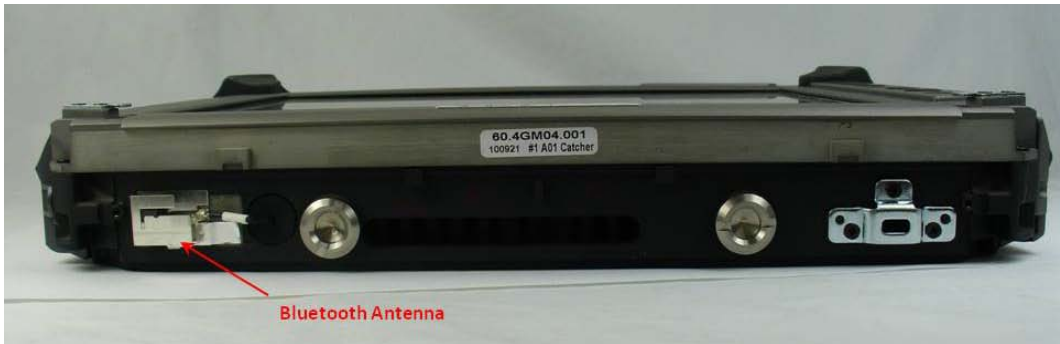
Figure 3 Bottom View – Bluetooth Antenna
