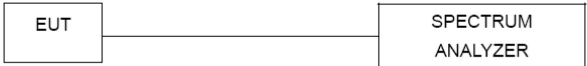
2. The bandwidth of the fundamental frequency was measure by spectrum analyser with 1MHz RBW and 1MHz VBW. The 20dB bandwidth is defined as the total spectrum the power of which is higher than peak power 20dB.
