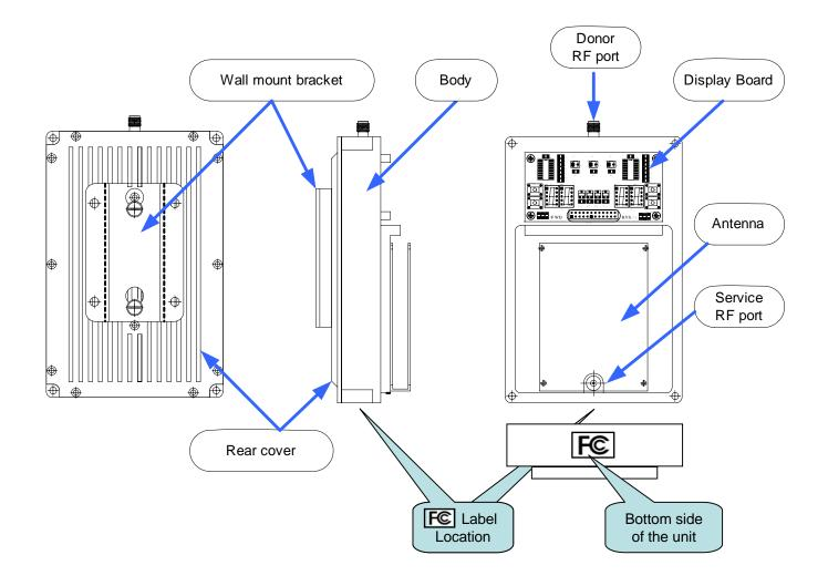
FCC label will be put on the bottom side of the repeater.
