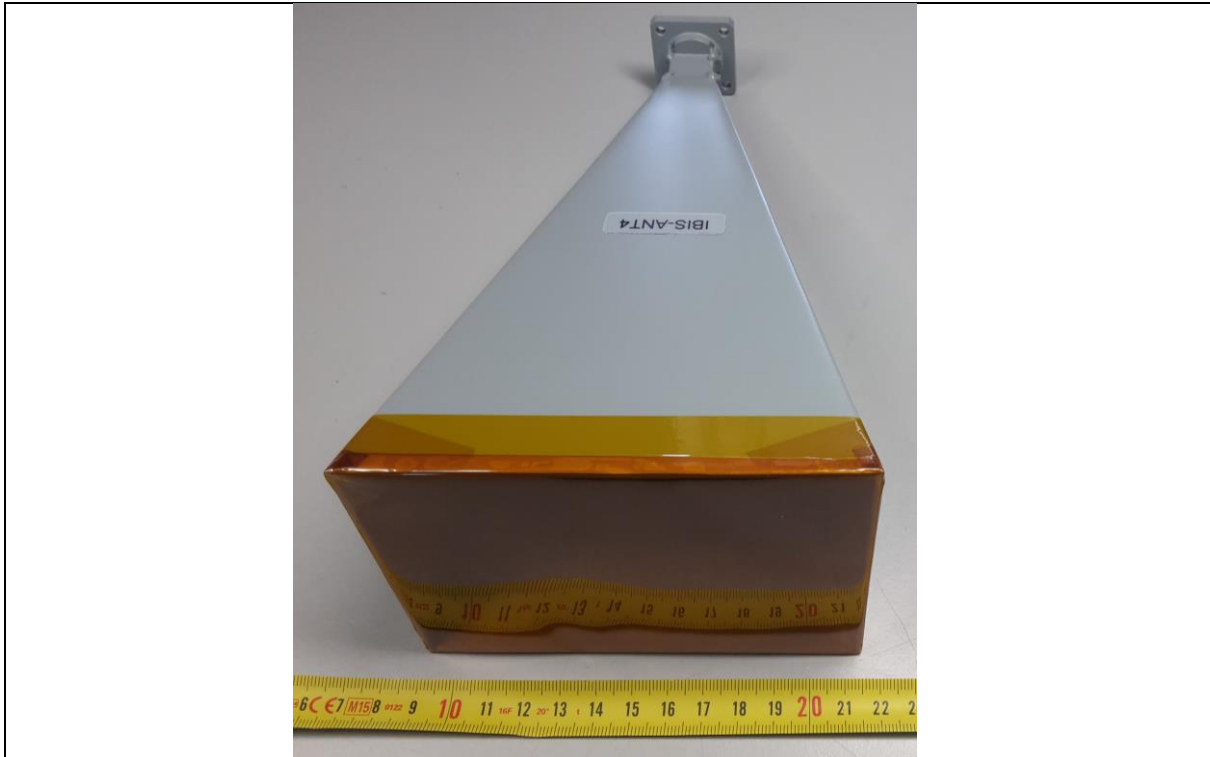
Antenna 4 (IBIS-ANT4-H11V10) – Front View
