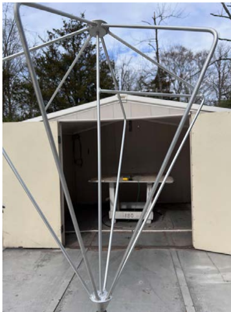
Figure 3.1 Radiated Emission Test Setup
