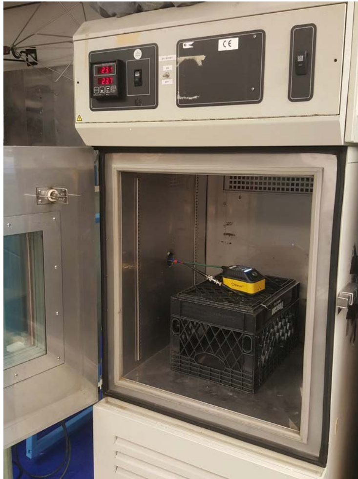
Figure 3.3 Frequency Tolerance Test Setup
