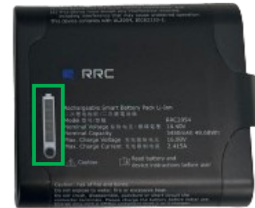
Fig. 65 Battery status check
