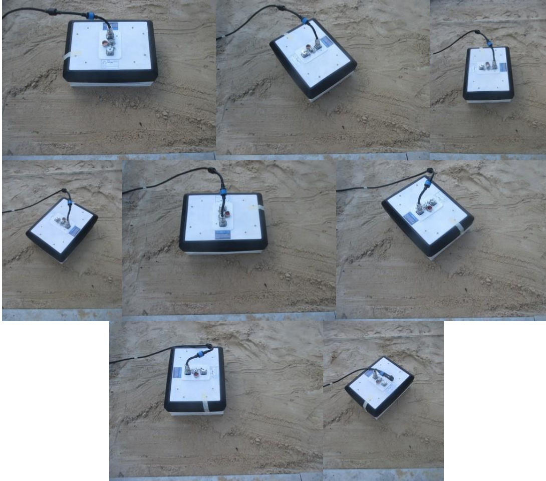
EUT Positions with 45 Degree Interval
