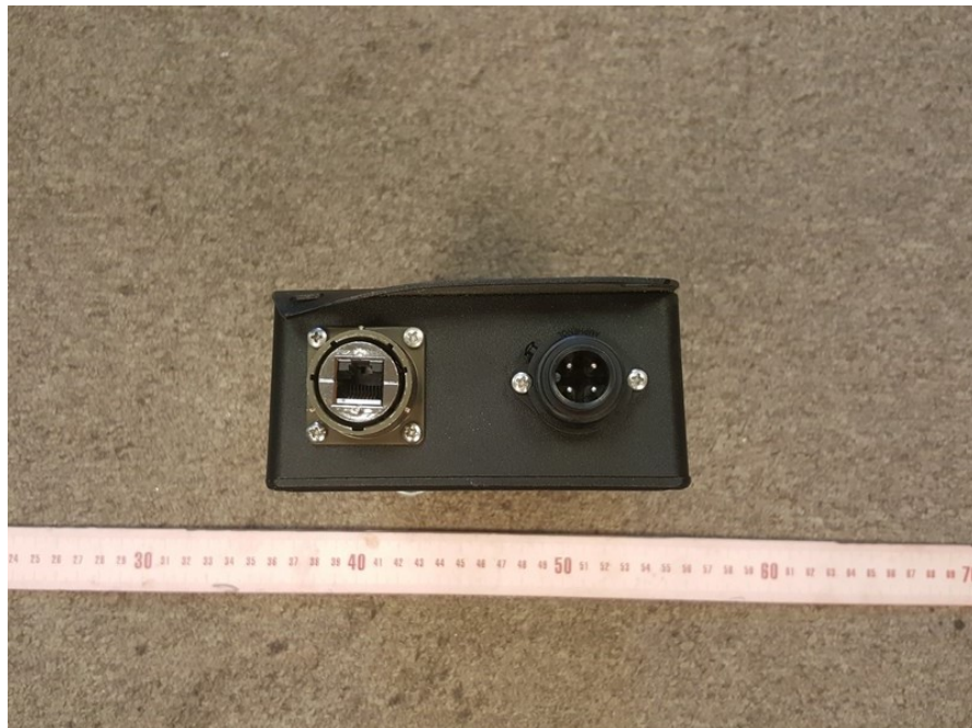
Cable Interface_ Network Port Side
