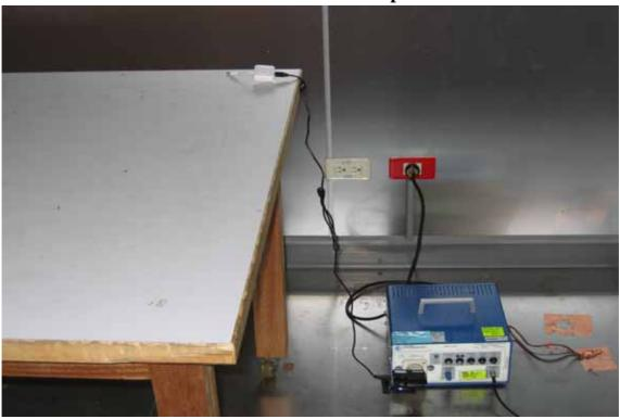
**Conducted Emission Set up Photo (Audio-in Mode)**
