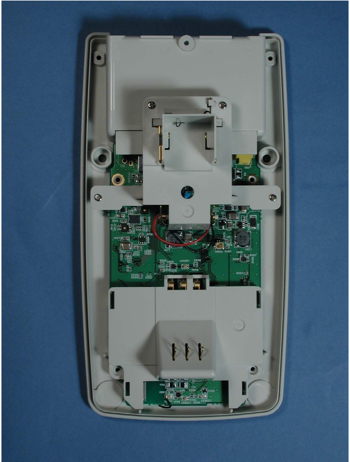
Photograph 9: - Cradle CRD-3101 inside view
