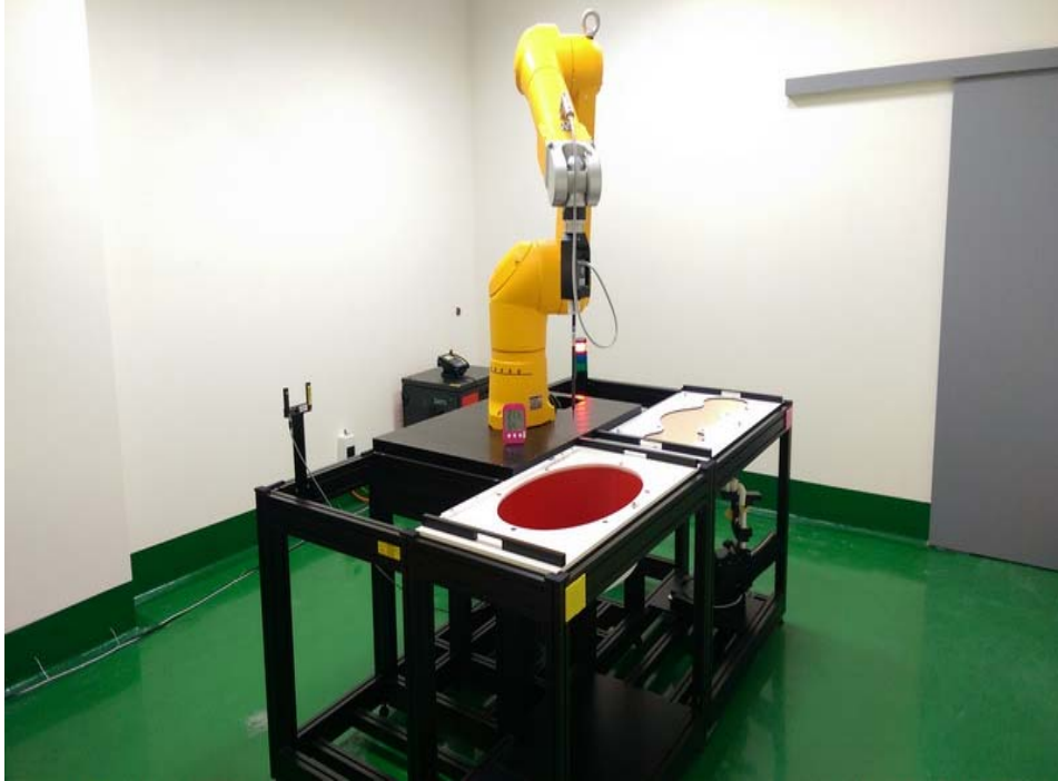
Liquid depth in the flat Phantom ( \geq 15\text{cm} depth) Body(2400MHz~2500MHz)
