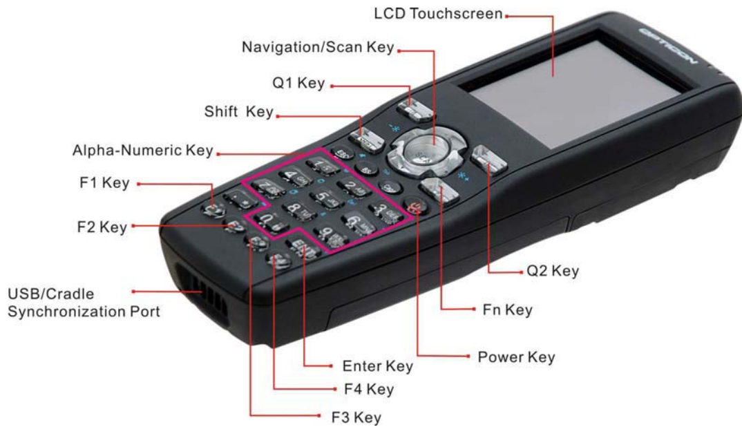
Figure 2-2 PDT front view
