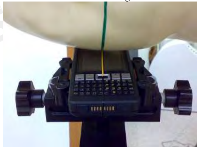
Fig.4 Right Head Section/ Ear-Tilt Position(15°)
