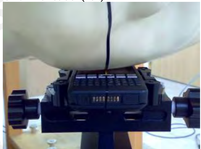
Fig.5 Left Head Section/ Cheek-Touch Position
