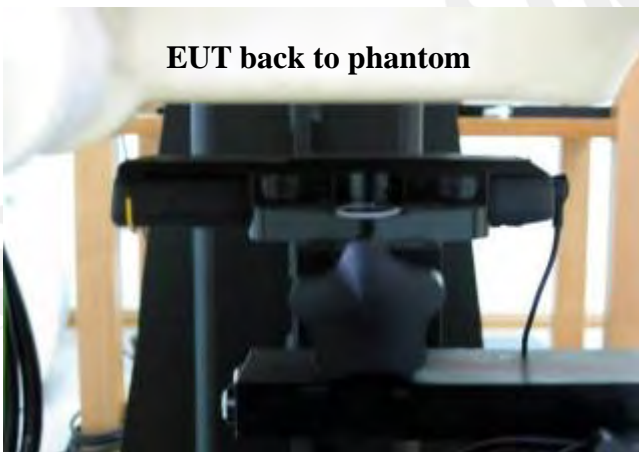
Fig.9 Body worn- EUT back to flat phantom and distance between flat phantom and mobile phone is 1.5 cm
