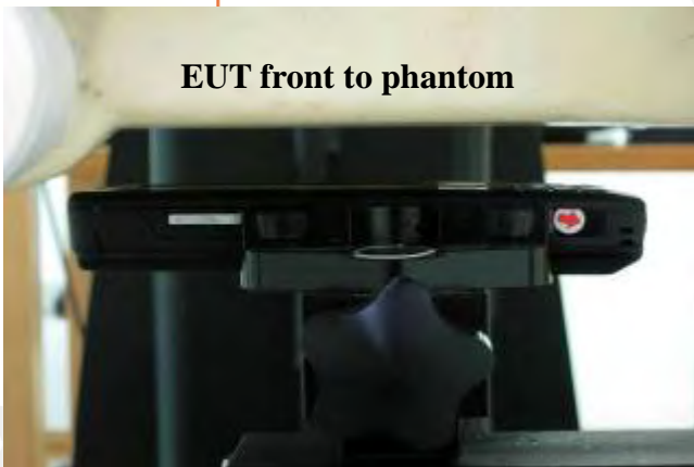
Fig.7 Body worn- EUT front to flat phantom and distance between flat phantom and mobile phone is 1.5 cm
