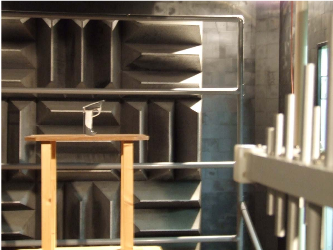
Photograph 1: Test setup Radiated Emissions (< 1 GHz) Scanner OPR-3101
