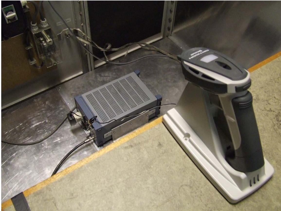
Photograph 3: Test setup Conducted Emissions Cradle CRD-3101
