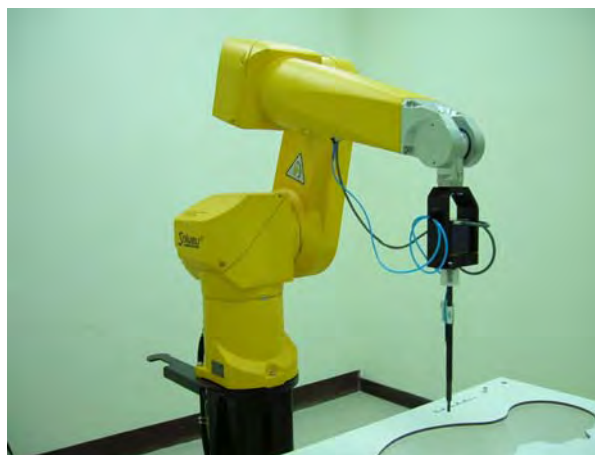
Fig. 5.2 Probe setup on robot
