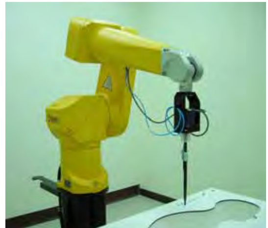
Fig. 5.2 Probe Setup on Robot
