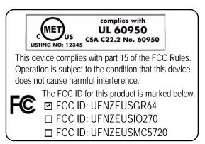
Proposed label for Zeus with Wavecom GR64 module.
