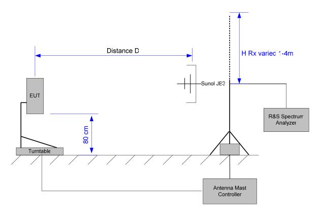
Note: Measurements below 1 GHz were performed with the Sunol JB3 antenna. Measurements above 1 GHz were performed with the Com-Power AHA-118 antenna. The measurement distance was 3 m.
