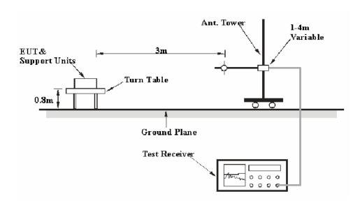
The radiated emission tests were performed in the 3 meters test site, using the setup accordance with the ANSI C63.4-2003. The related limit was specified in FCC Part 15.109.
