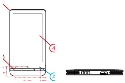
Center Button: Press and hold for 5 seconds -On/ Off, Press and hold for 10 seconds -reset,
