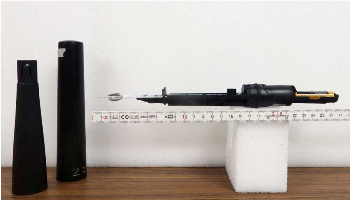
Side View – Antenna PCB & Battery Exposed 90 degrees
