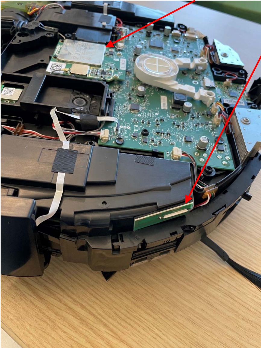
Photo 15 – Roomba Combo j7, Model RCA-Y1 Sextant Module external antenna location:
