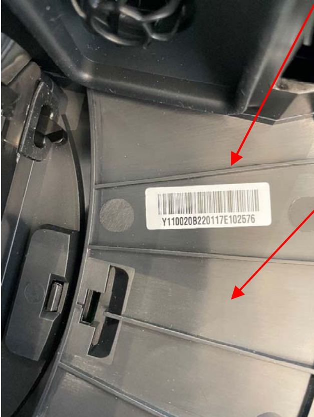
Photo 7 – Roomba Combo j7, Model RCA-Y1 Serial Number and the laser etch product label will go under the serial number. See artwork label file in separate document:
