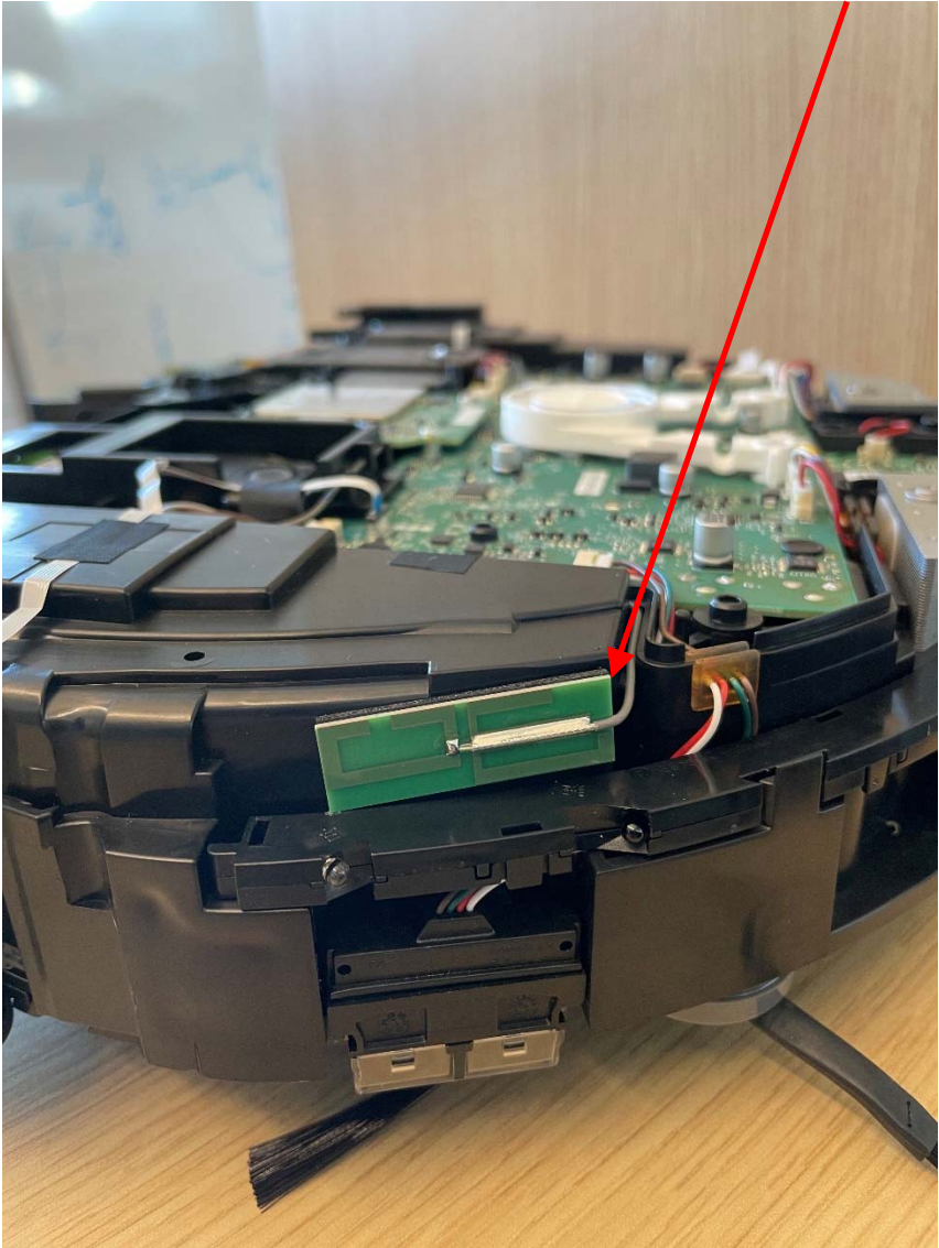
Photo 14 – Roomba Combo j7, Model RCA-Y1 Sextant Module external antenna location:
