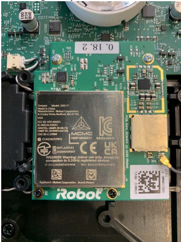
Photo 13 – Roomba Combo j7, Model RCA-Y1 closeup of Sextant Radio Module Model AXG-Y1 etched Regulatory Label:
