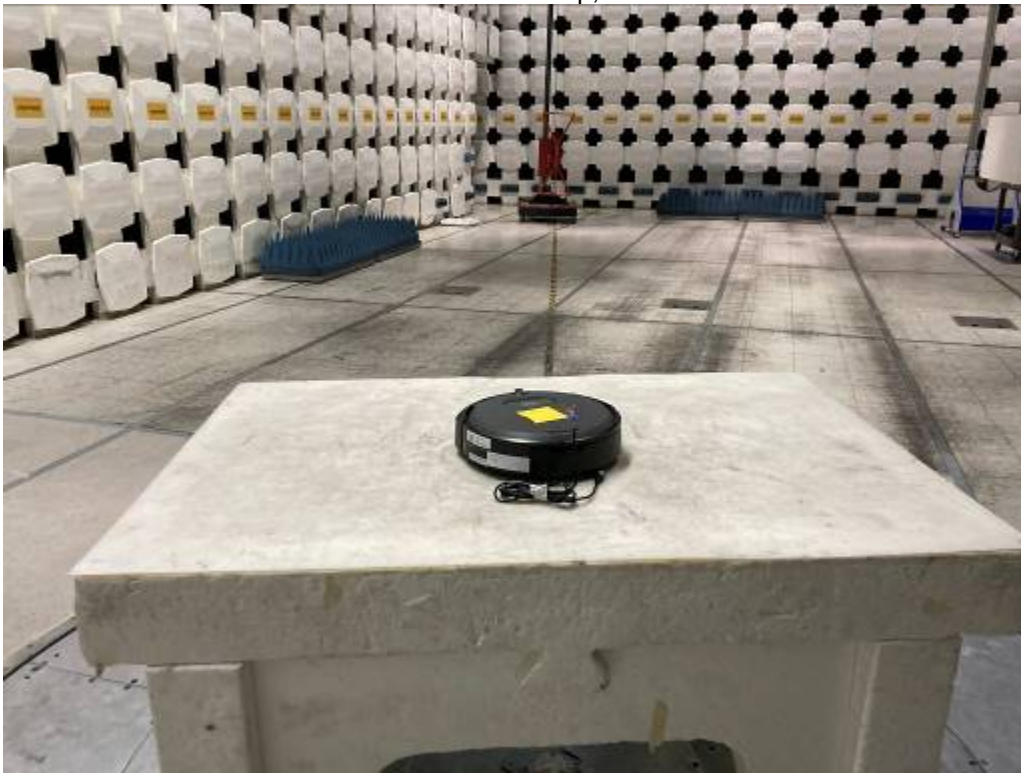
Radiated Emissions Test Setup, Below 1000 MHz
