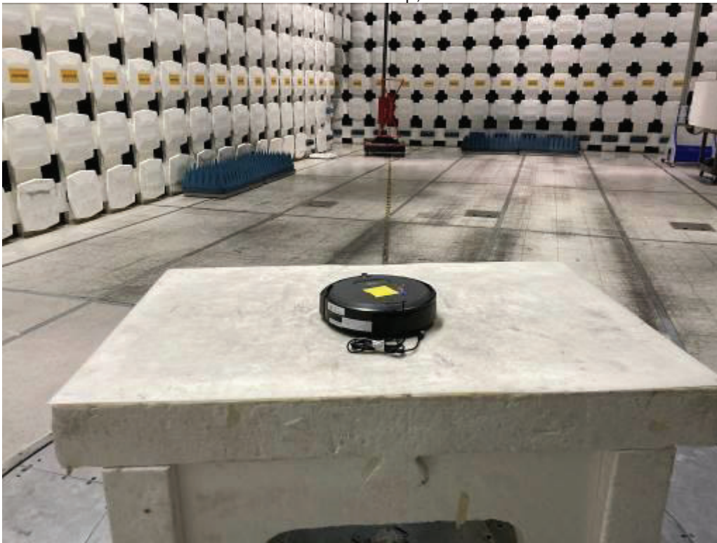
Radiated Emissions Test Setup, Below 1000 MHz
