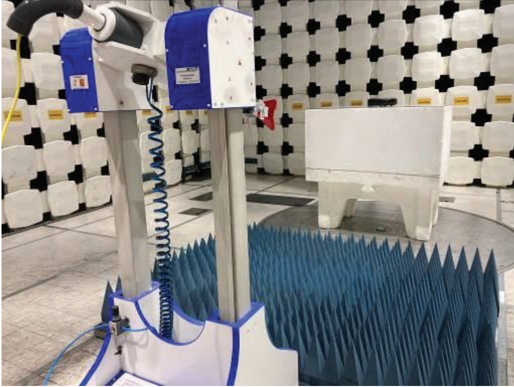
Radiated Emissions Test Setup, 1-18 GHz
