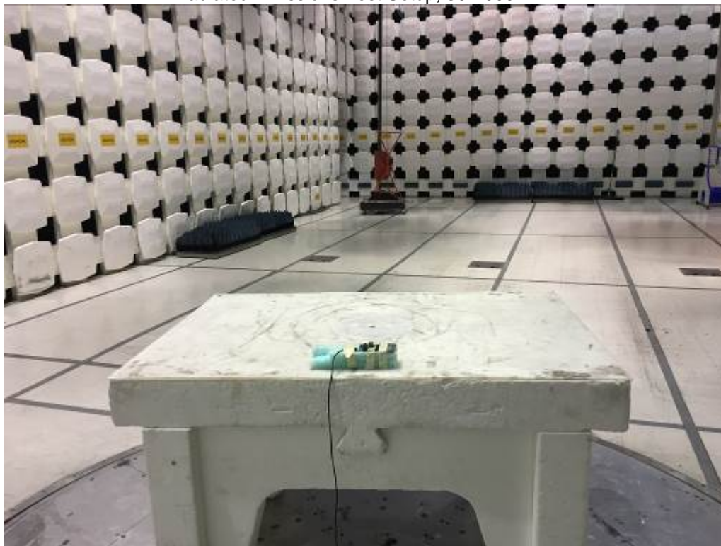
Radiated Emissions Test Setup, 30-1000 MHz
