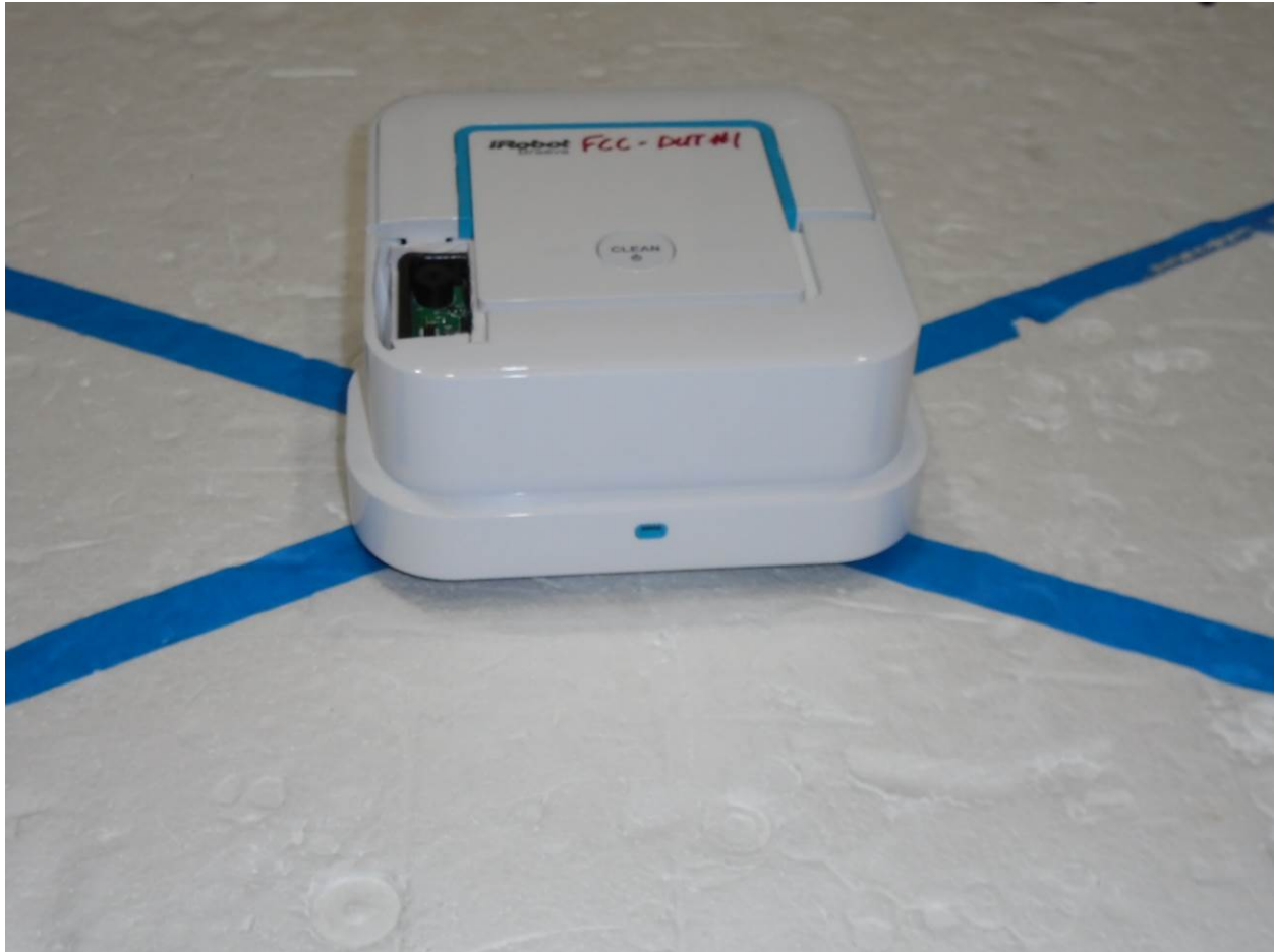
Figure 5: Radiated Emissions – Orientation A Investigation for highest emissions Note: Orientation A provided the highest emissions
