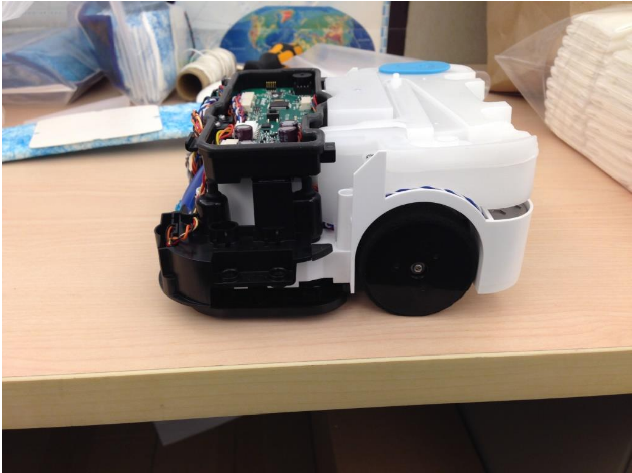
Figure 2: Side internal View. (Photo provided by iRobot)
