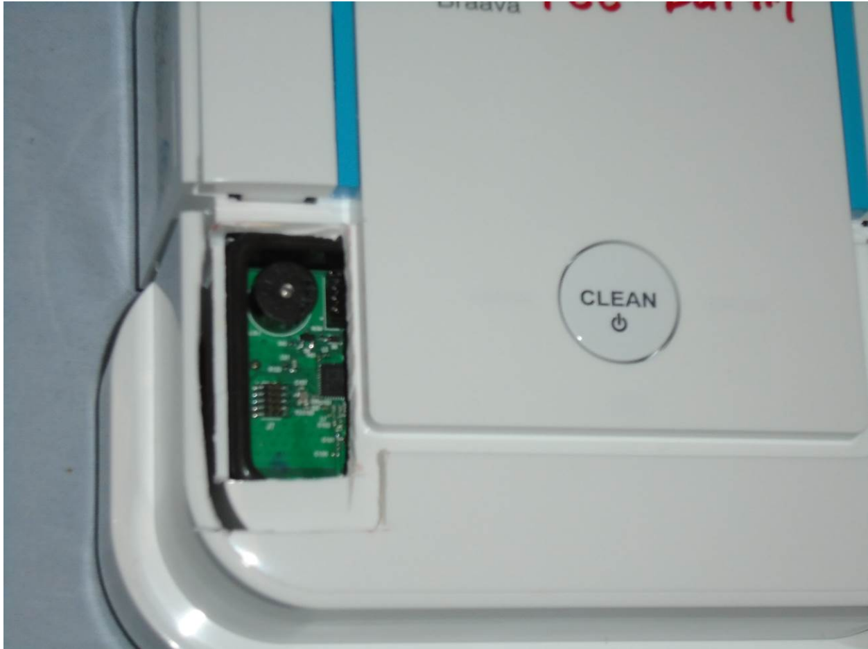
Figure 5: View of EUT with case modified to allow access to the programming port.
