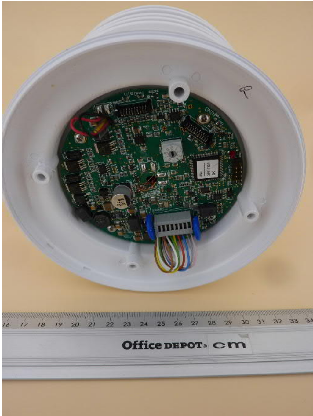
WS700-UMB housing with main PCB, shielding removed
