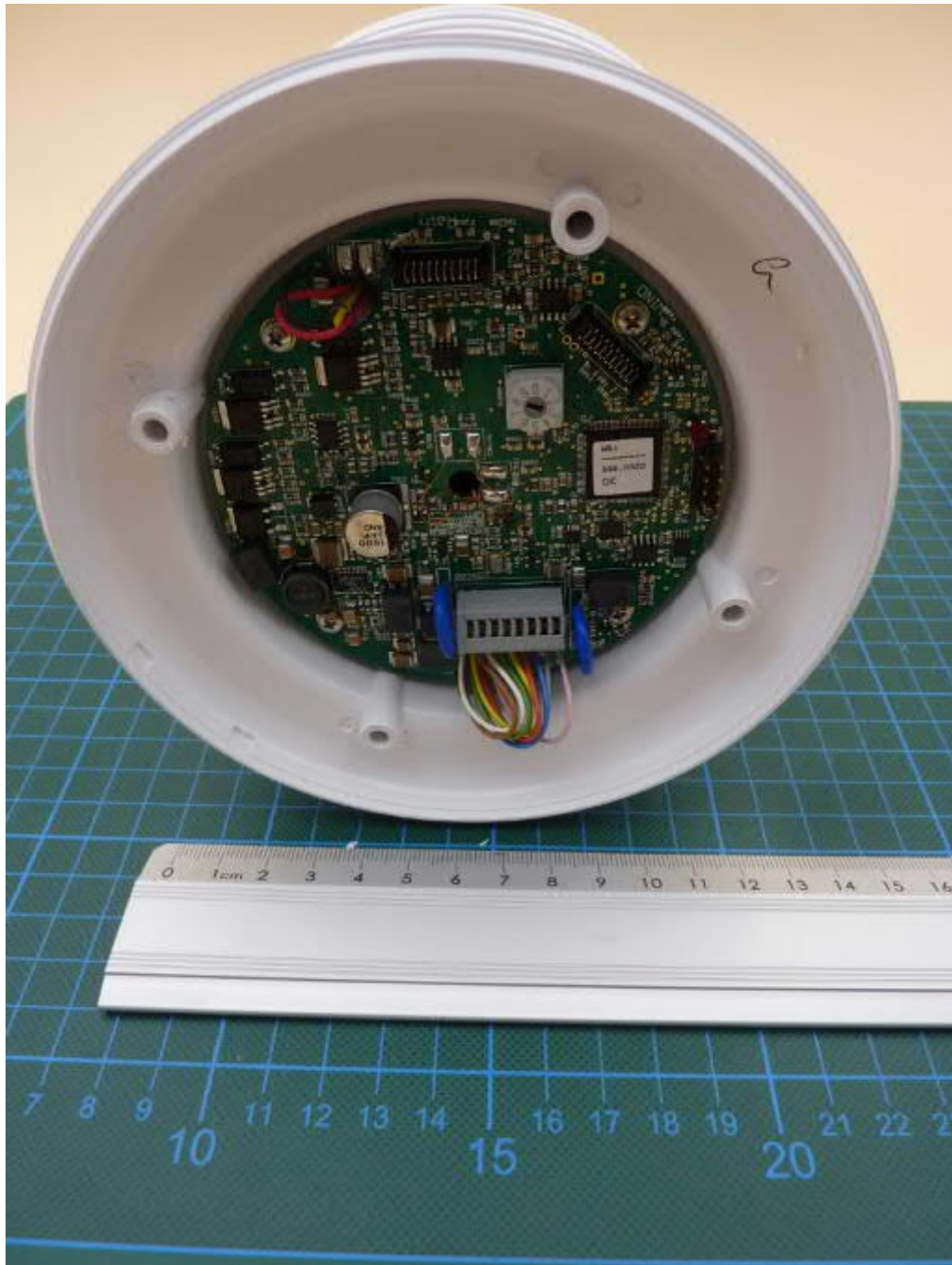
WS600-UMB housing with main PCB, shielding removed
