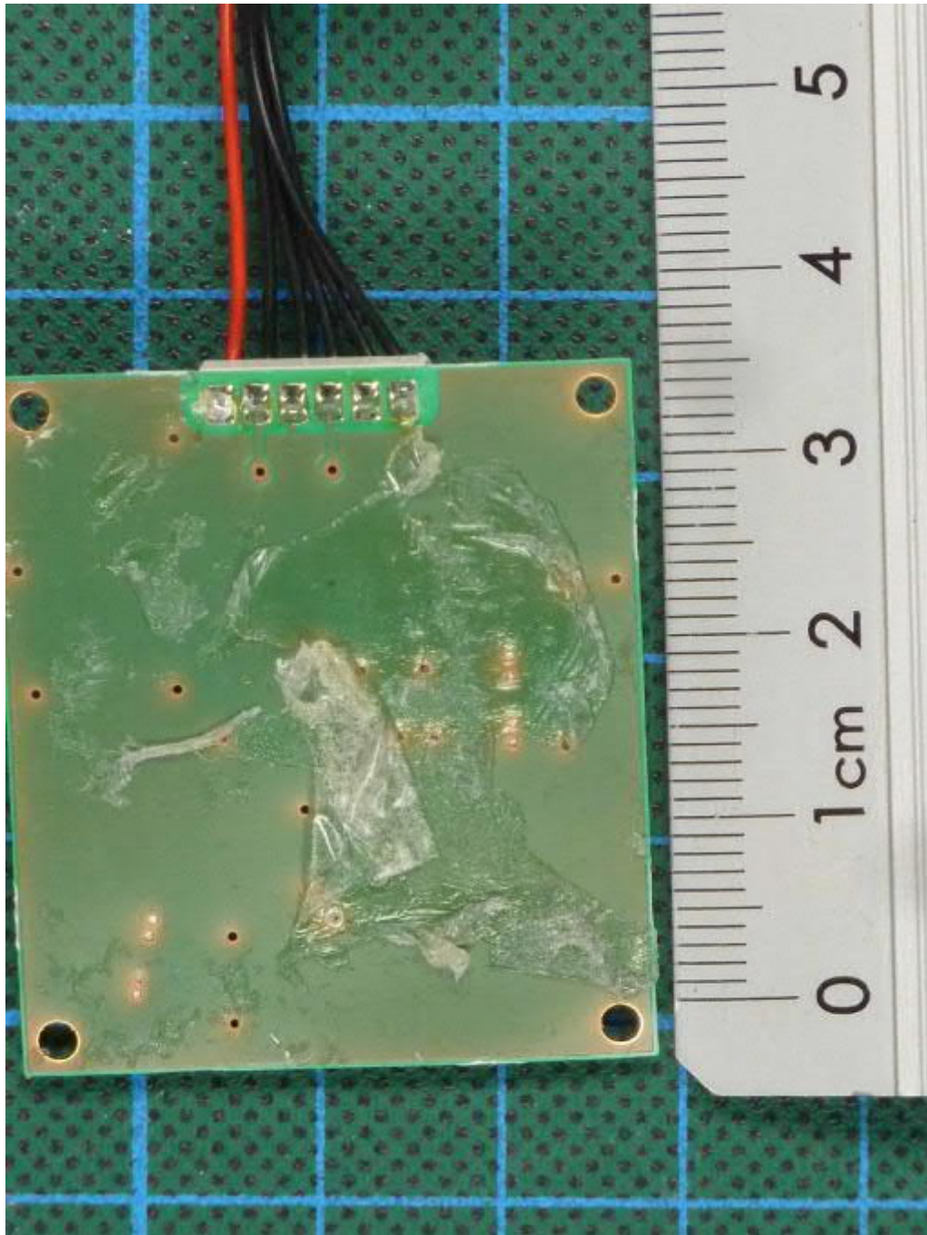
WS400-UMB, radar module, PCB, bottom view
