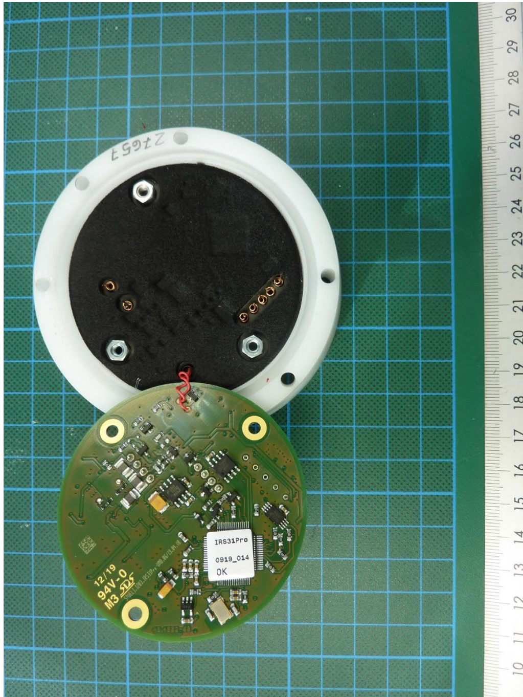
IRS31Pro-UMB, PCB, bottom view
