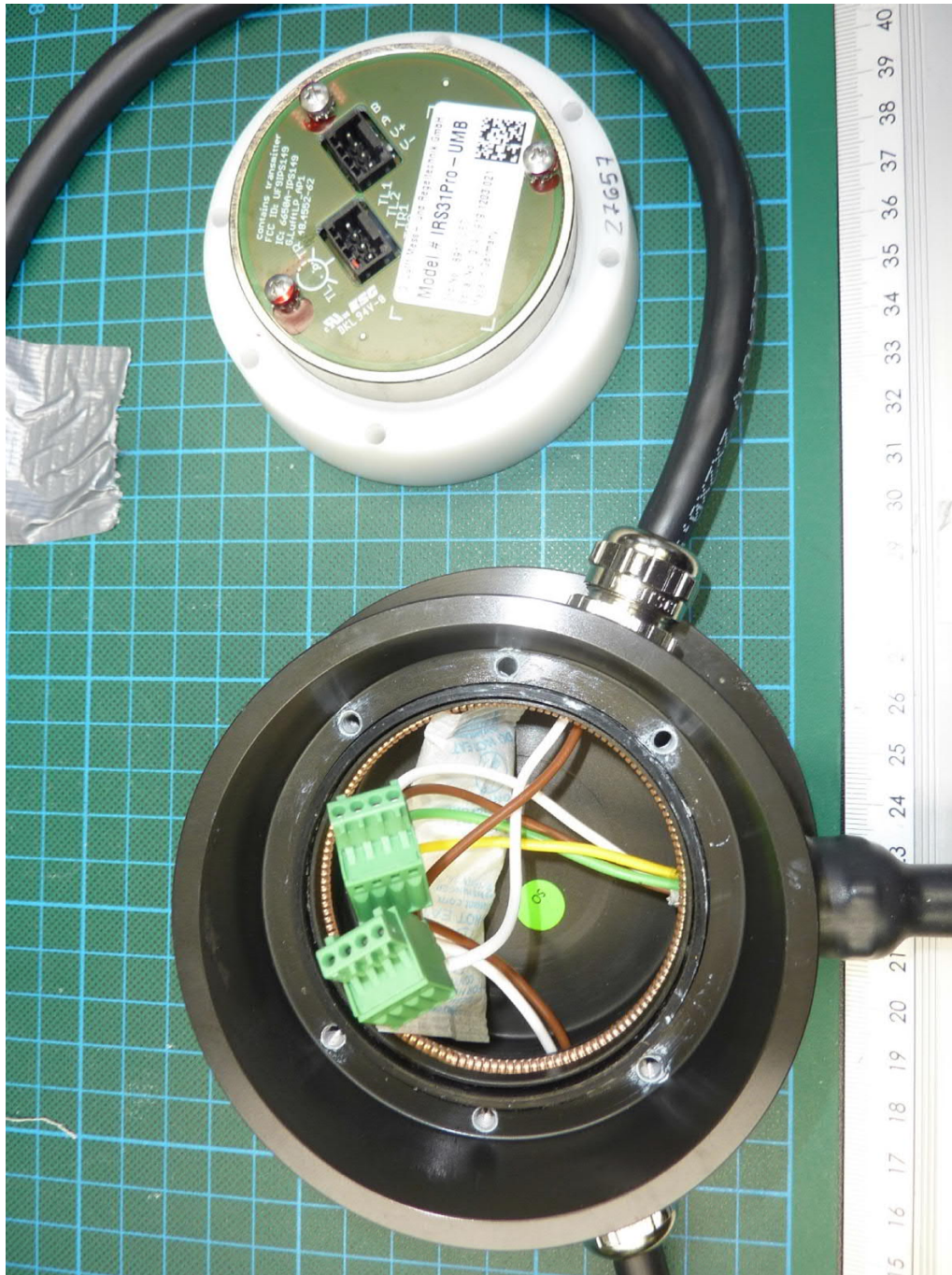
IRS31Pro-UMB, internal view (electronic disconnected)
