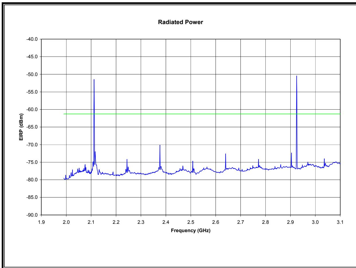
The narrowband emissions over the UWB limit were identified as emissions from digital circuitry used to enable the operation of the UWB transmitter, and are not intended to be radiated from the transmitter's antenna.
