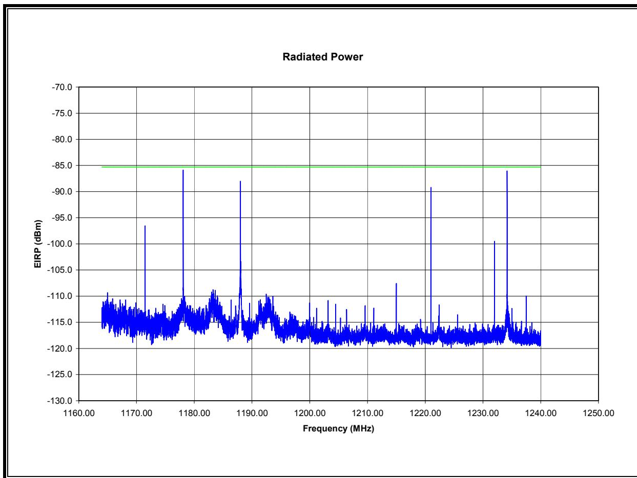
**EIRP 1.164 TO 1.240 GHz, 1 kHz BW, VERTICAL**
