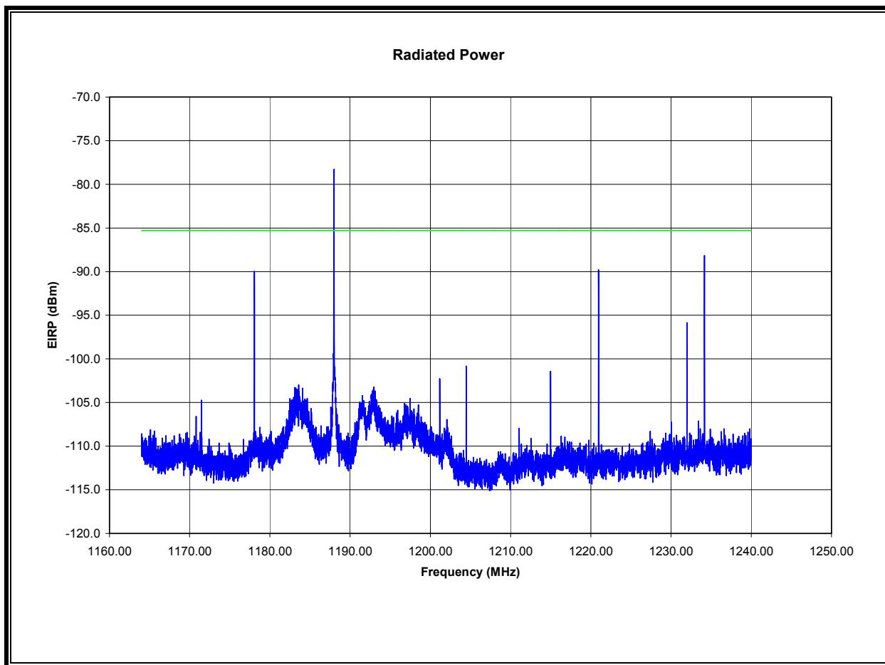
Note: The narrowband emission over the UWB limit was identified as an emission from digital circuitry used to enable the operation of the UWB transmitter, and is not intended to be radiated from the transmitter's antenna.
