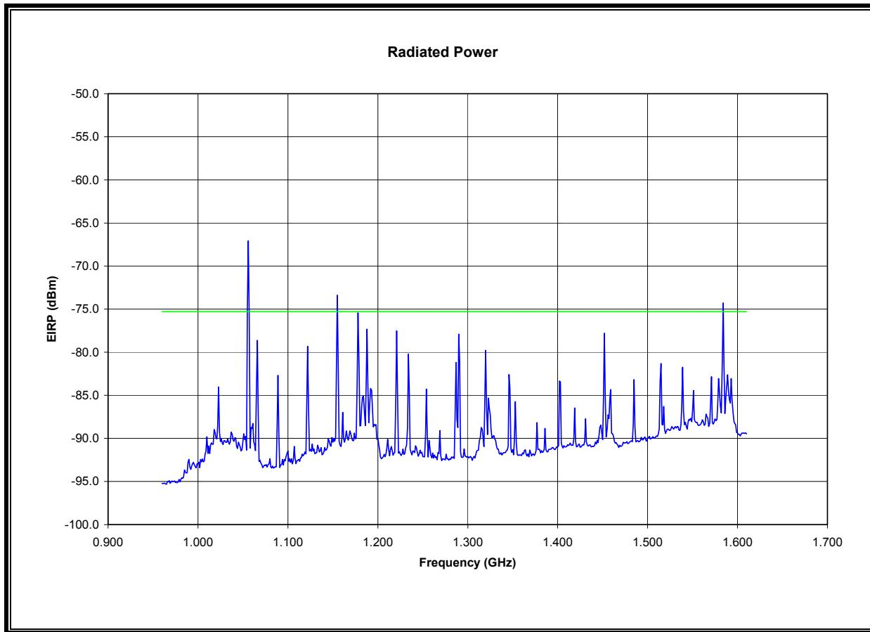
Note: The narrowband emissions over the UWB limit were identified as emissions from digital circuitry used to enable the operation of the UWB transmitter, and are not intended to be radiated from the transmitter's antenna.
