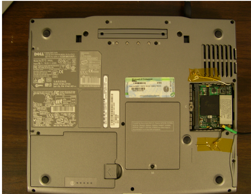
Figure 1. Tzero TZ7110 Mini-PCI adaptor mounted in laptop.
