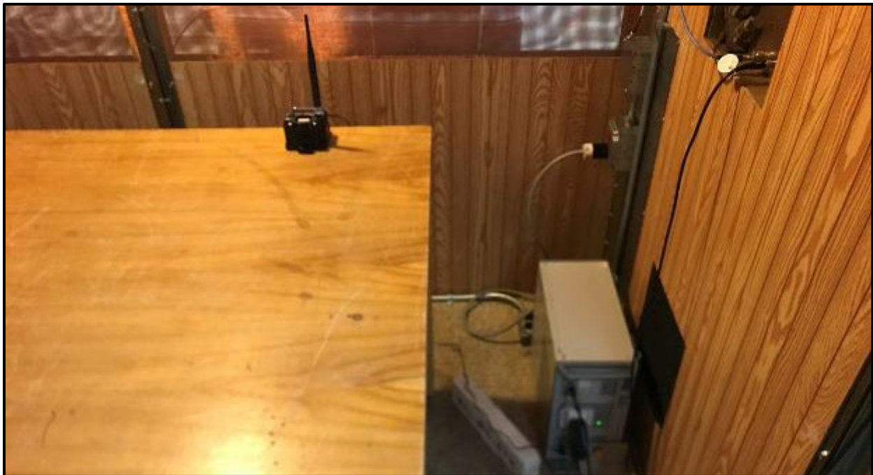
Figure 2-1: Configuration of Tested System, Conducted Emissions
