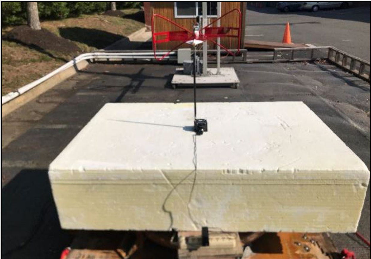
Photograph 6: Radiated Emissions Test Setup <1 GHz, 5 dBi Monopole, Rear
