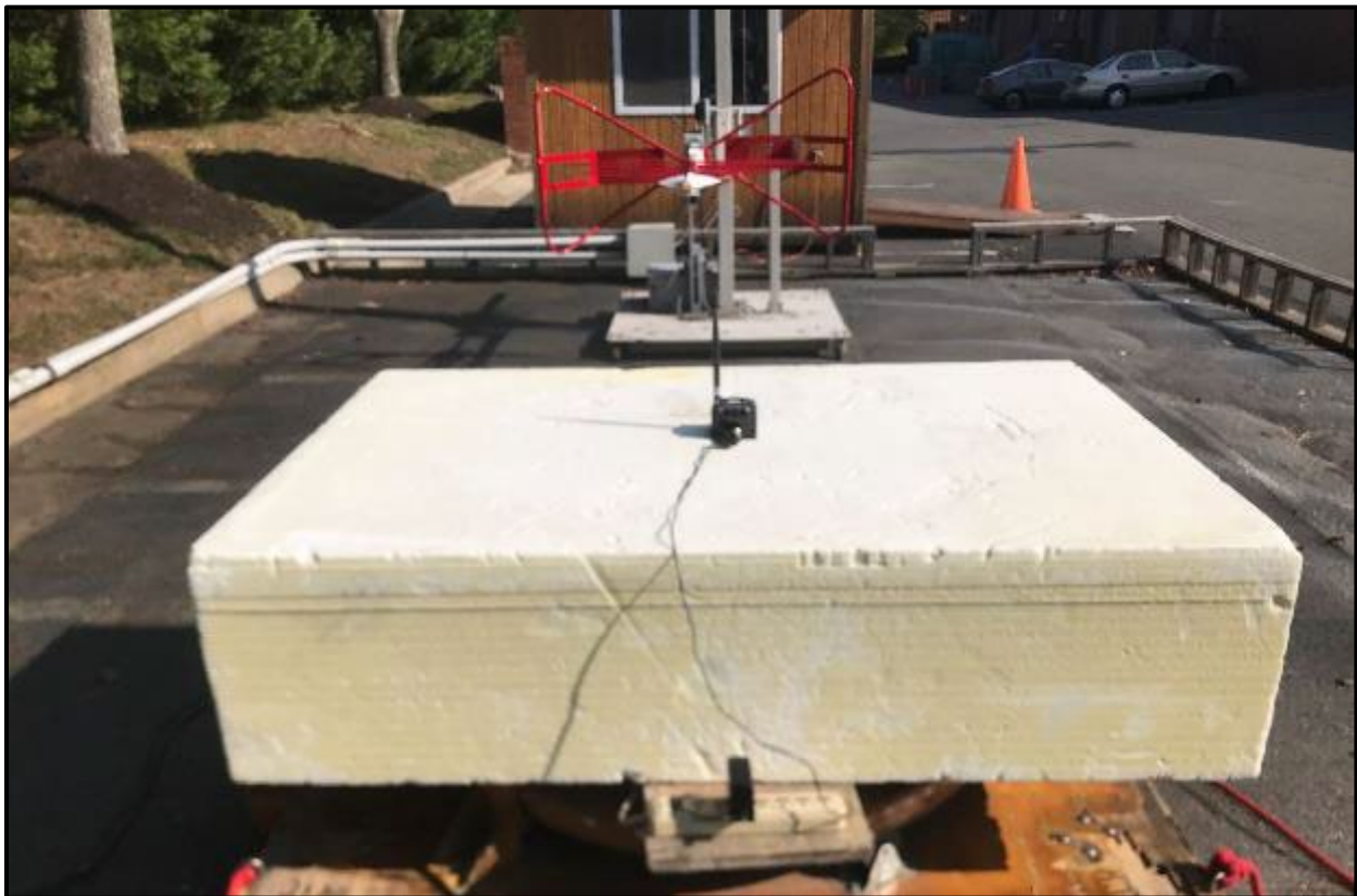
Photograph 4: Radiated Emissions Test Setup <1 GHz, 2 dBi Monopole, Rear
