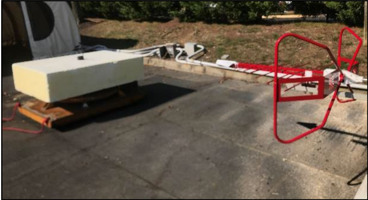
Photograph 3: Radiated Emissions Test Setup <1 GHz, 2 dBi Monopole, Front
