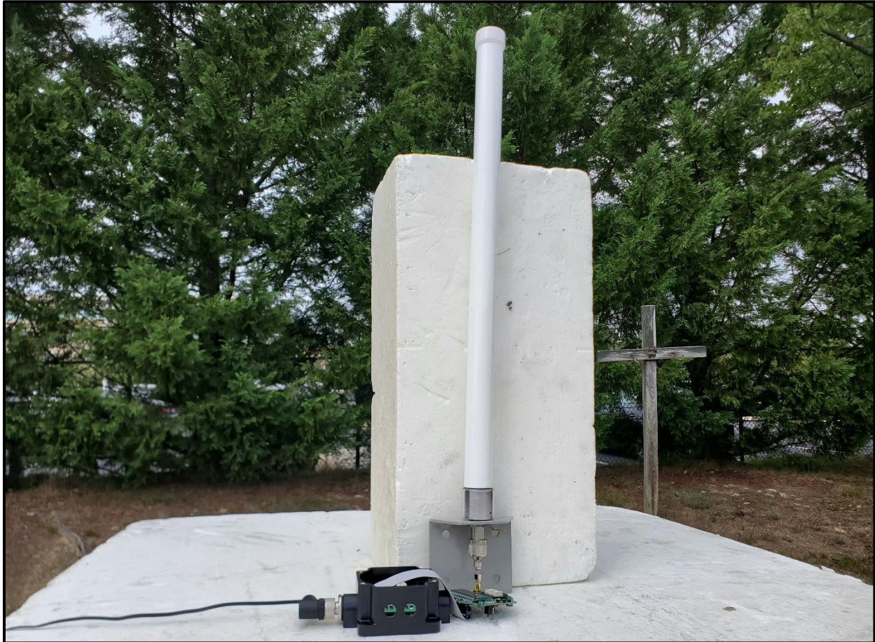
Photograph 17: Radiated Emissions Test Setup >1 GHz, 6 dBi Dipole, Stand-alone
