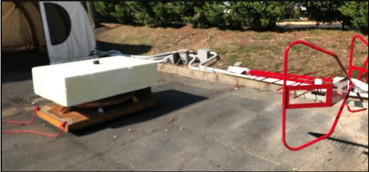
Photograph 5: Radiated Emissions Test Setup <1 GHz, 5 dBi Monopole, Front
