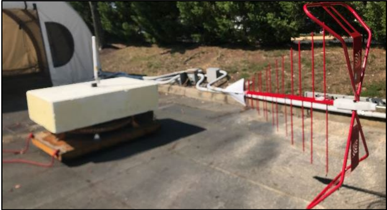
Photograph 7: Radiated Emissions Test Setup <1 GHz, 6 dBi Dipole, Front
