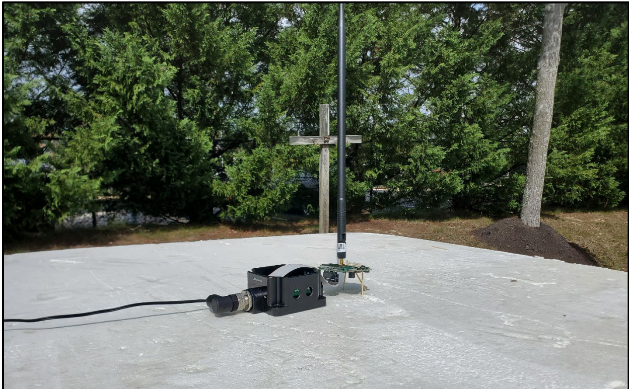
Photograph 16: Radiated Emissions Test Setup >1 GHz, 5 dBi Monopole, Stand-alone
