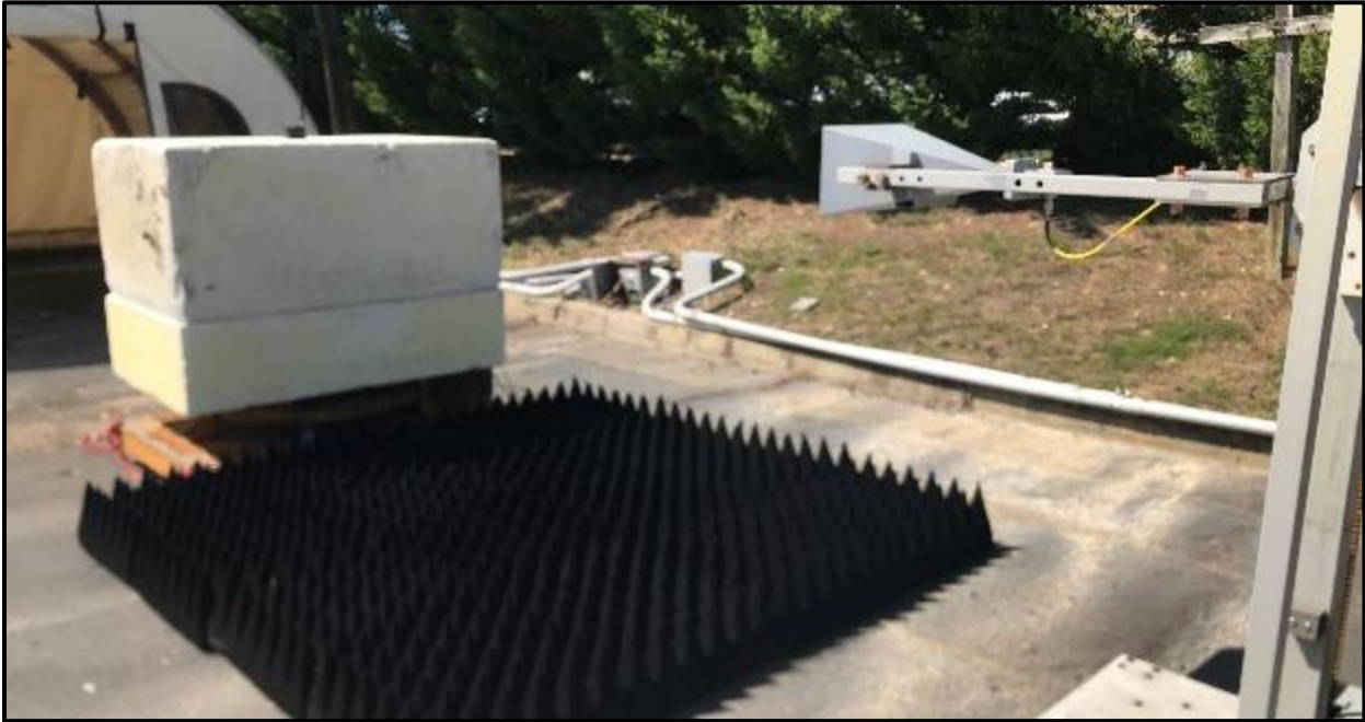
Photograph 11: Radiated Emissions Test Setup >1 GHz, 5 dBi Monopole, Front
