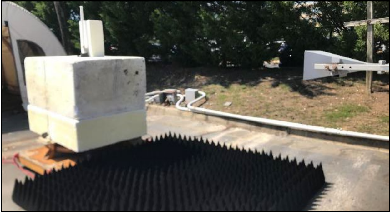
Photograph 13: Radiated Emissions Test Setup >1 GHz, 6 dBi Dipole, Front
