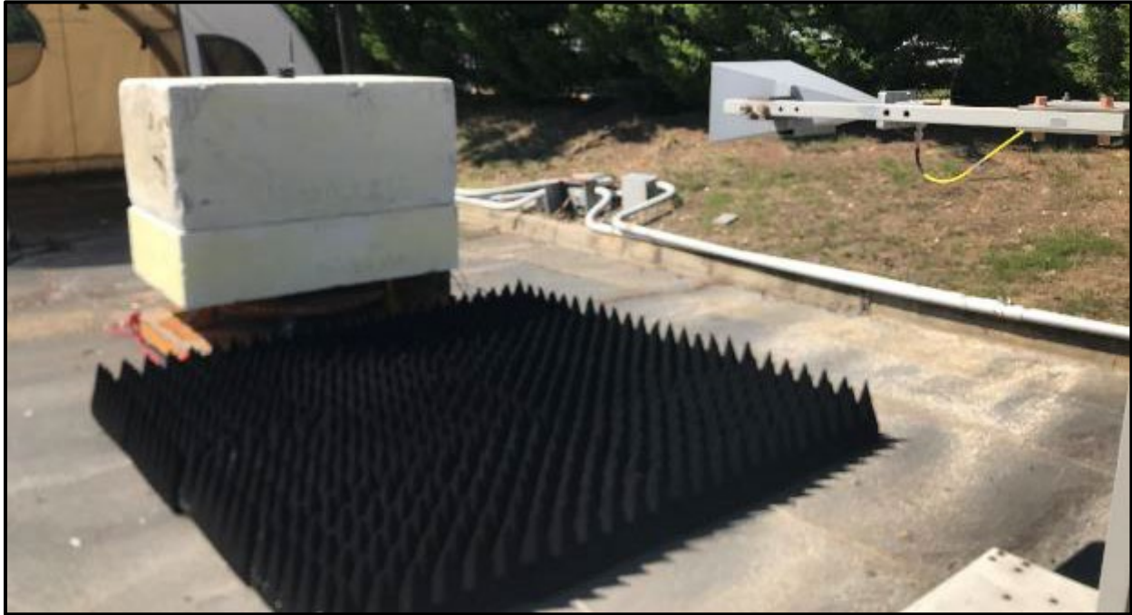
Photograph 9: Radiated Emissions Test Setup >1 GHz, 2 dBi Monopole, Front
