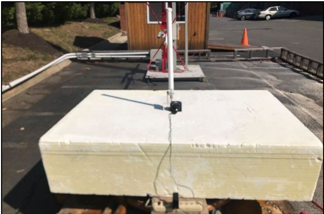
Photograph 8: Radiated Emissions Test Setup <1 GHz, 6 dBi Dipole, Rear
