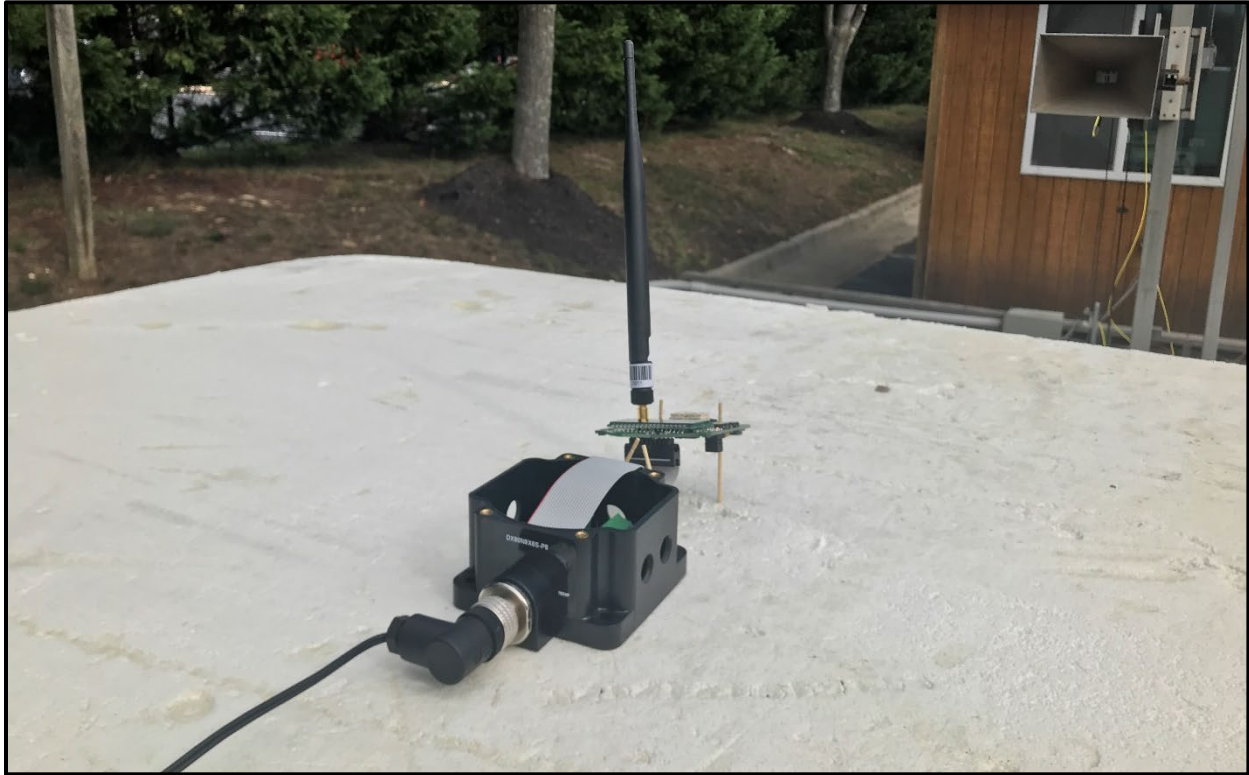
Photograph 15: Radiated Emissions Test Setup >1 GHz, 2 dBi Monopole, Stand-alone
