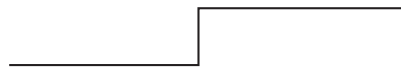
With a debounce filter, the signal is interpreted to change state only once.
