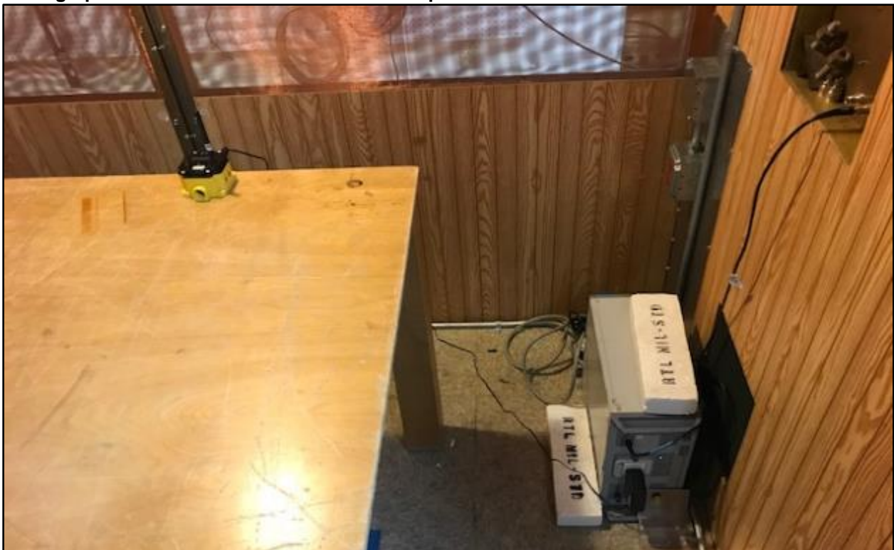
Photograph 4: Conducted Emissions Test Setup
