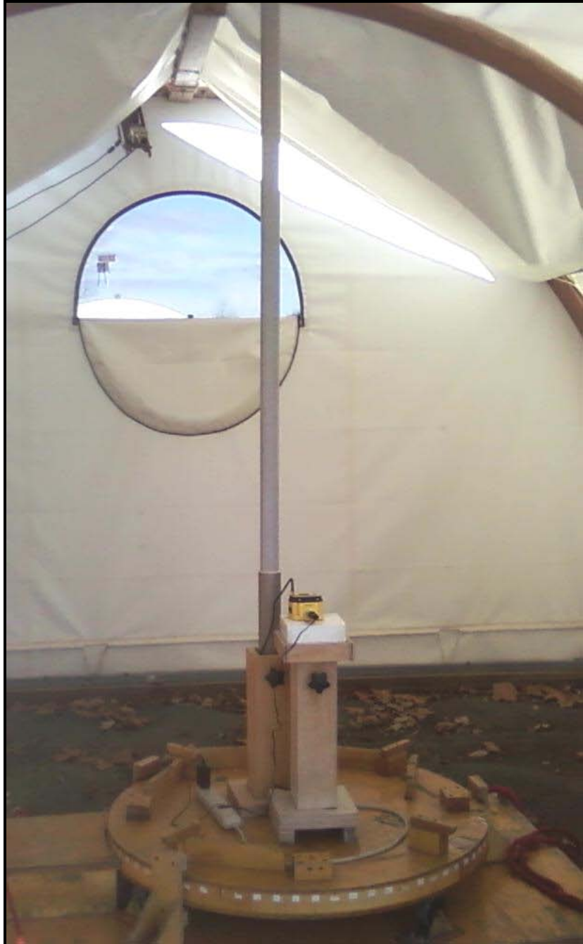
Photograph 5: Radiated Emissions Testing – Back View 8dBi Dipole Antenna with Host
