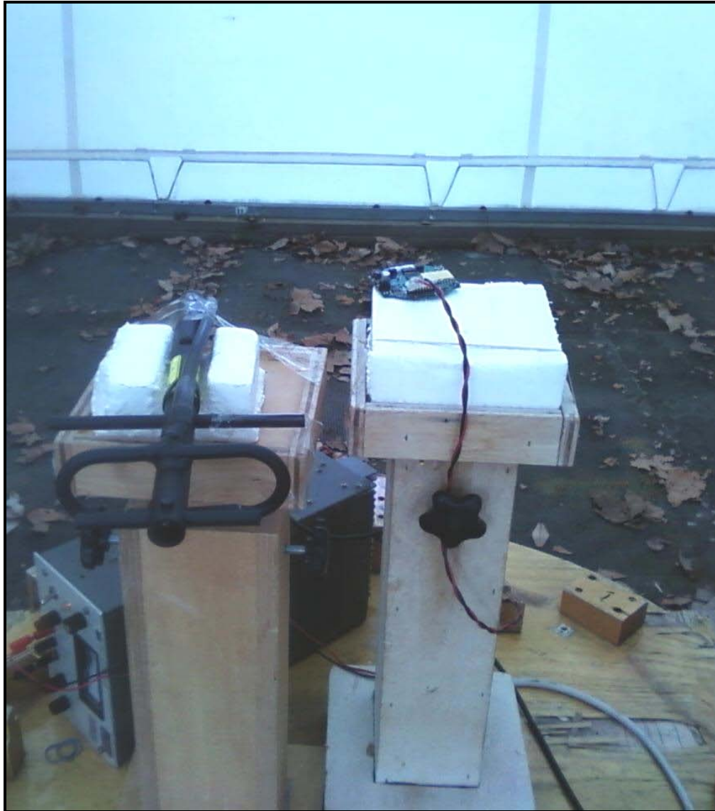
Photograph 14: Radiated Emissions Testing – Front View 6dBi Yagi Antenna with Module
