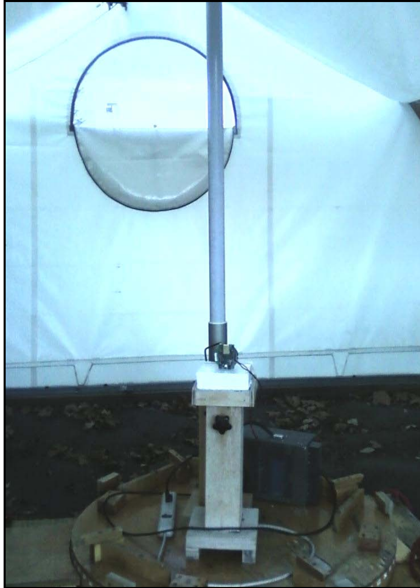
Photograph 10: Radiated Emissions Testing – Front View 8dBi Dipole Antenna with Module
