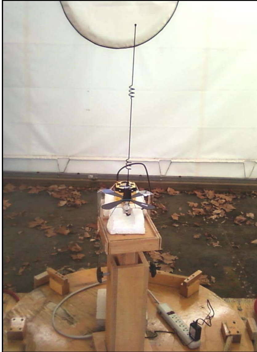
Photograph 6: Radiated Emissions Testing – Front View 5dBi Monopole Antenna with Host
