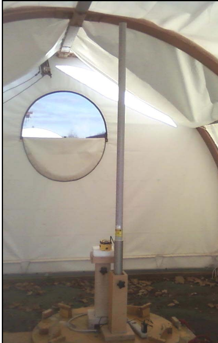
Photograph 4: Radiated Emissions Testing – Front View 8dBi Dipole Antenna with Host
