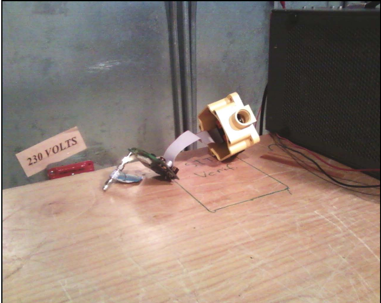
Photograph 16: Conducted Emissions Testing – Front View - Module
