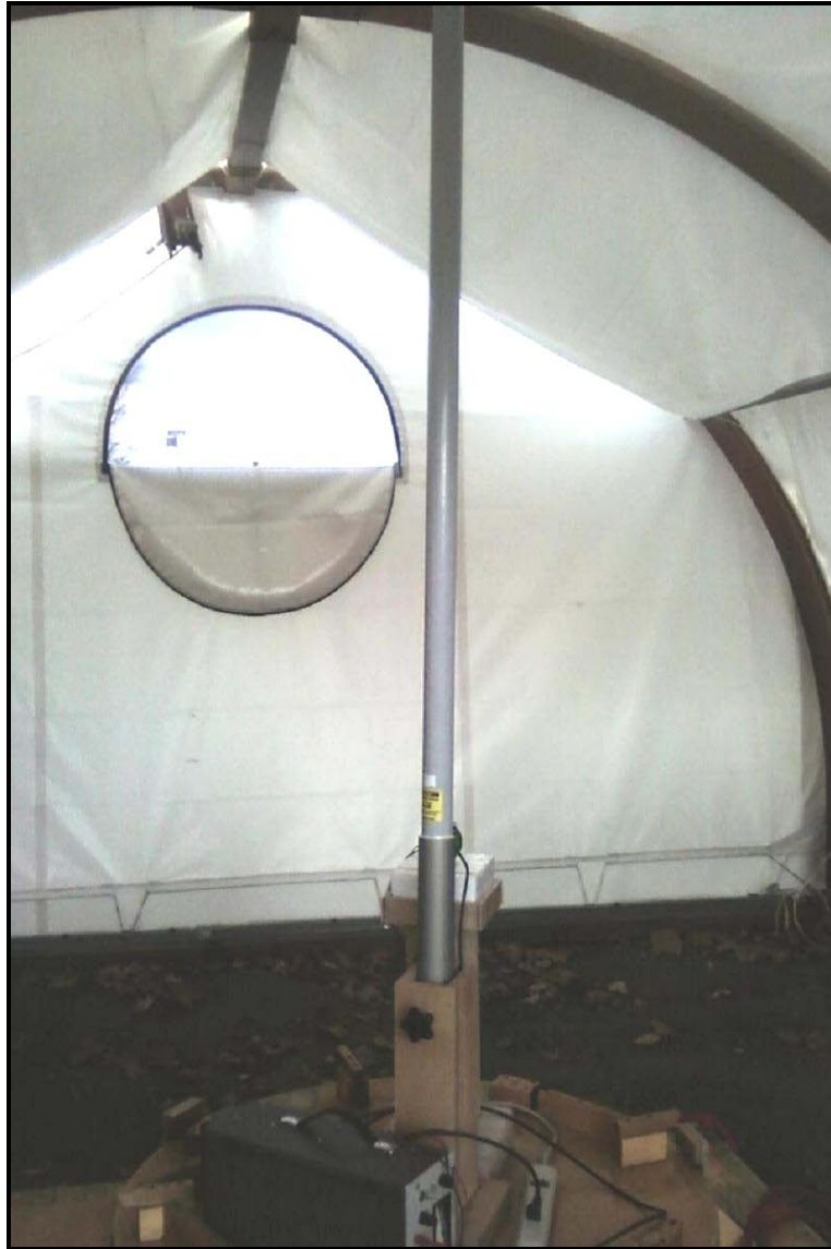
Photograph 11: Radiated Emissions Testing – Back View 8dBi Dipole Antenna with Module
