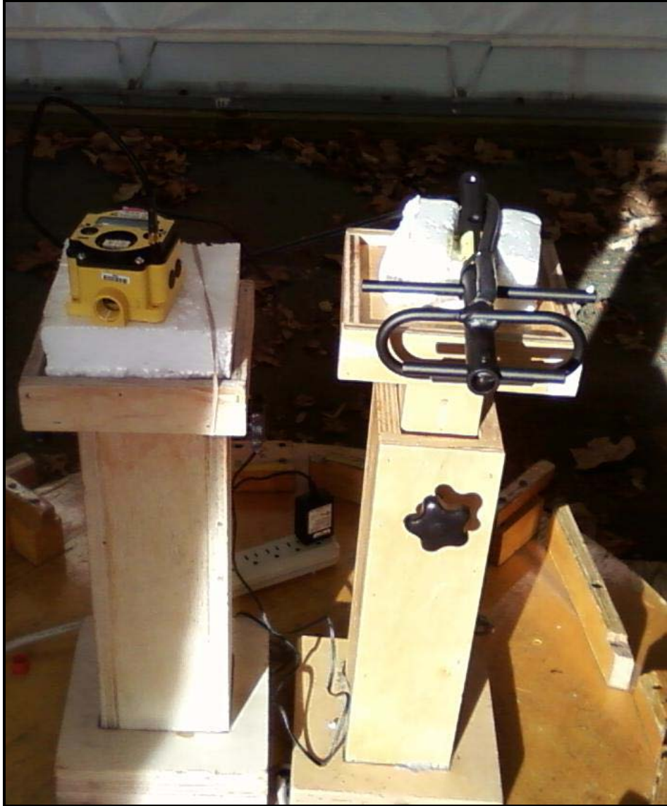
Photograph 8: Radiated Emissions Testing – Front View 6dBi Yagi Antenna with Host
